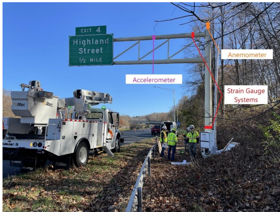
Figure 2.12. Sensor Types and Locations
