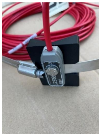
Figure 2.11. Accelerometer Attached to Band Clamp
