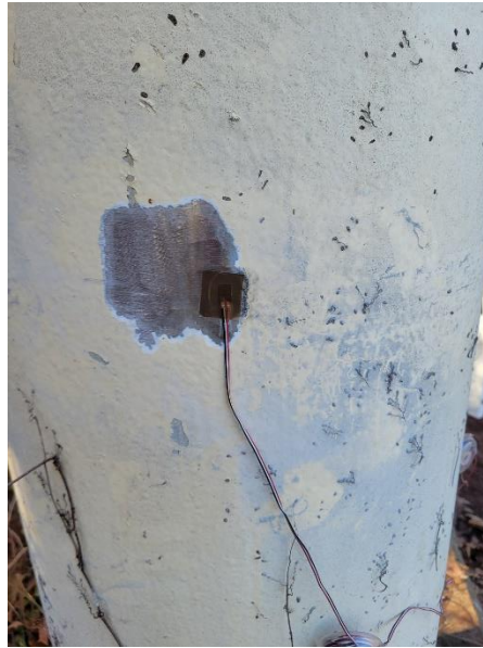
Figure 2.10. Typical Strain Gauge Installation
