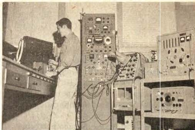
Clyde Scott, Avionics Technician at work on the laboratory test bench designed for checking Distance Measuring Equipment (DME).
