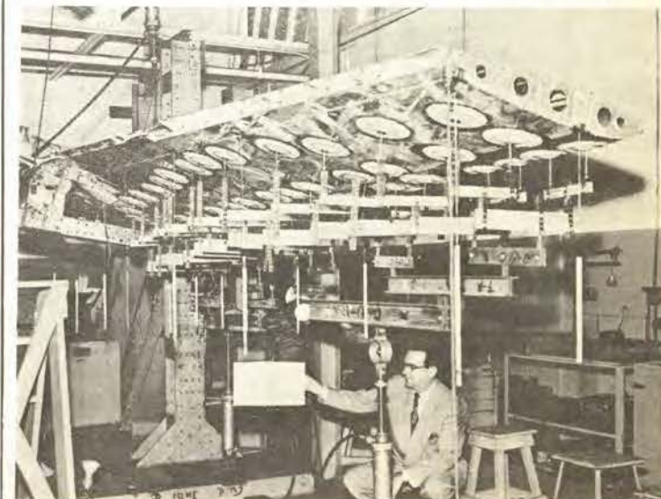
Whiffletree arrangement transmitting the load from hydraulic jacks to wing section.
