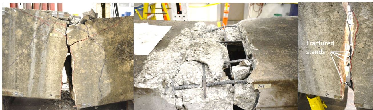
Figure 8. Photo. Failed G1 beam specimen.
