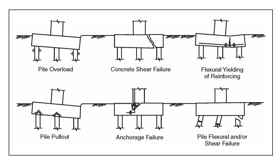
Figure D-12. Modes of failure for pile footings.
