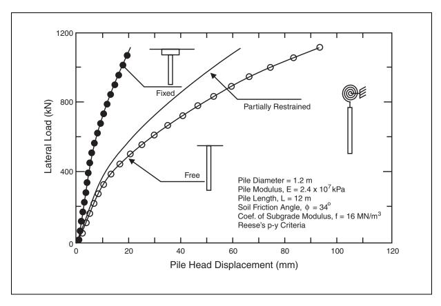
Figure 6-7. Effect of boundary conditions on pile stiffness
