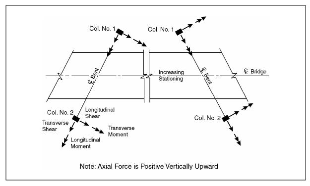
Figure E-5. Positive sign convention for column forces and moments.
