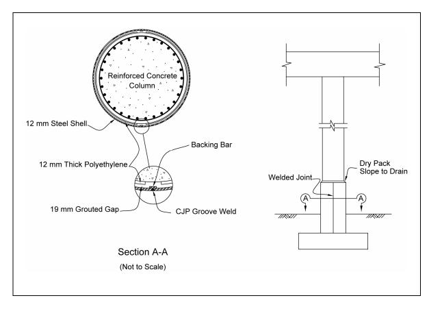
Figure 9-19. Steel shell retrofit for vertical capacity preservation.
