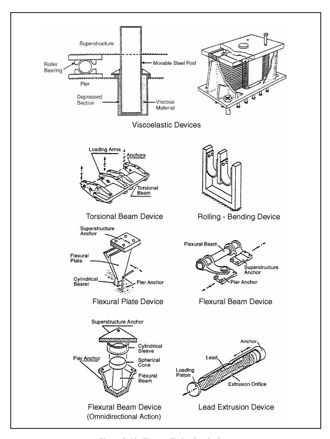
Figure 8-49. Energy dissipation devices.
