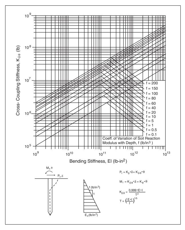
Figure 6-10. Cross-coupling pile-head stiffness.
