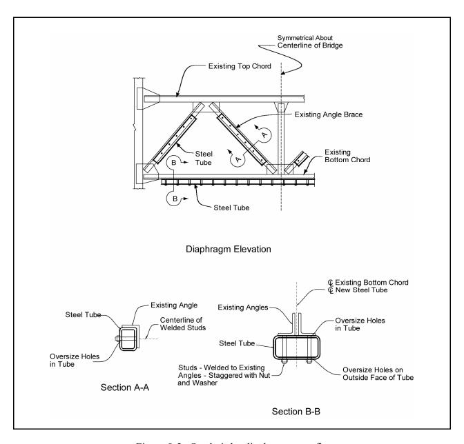
Figure 8-2. Steel girder diaphragm retrofit.
