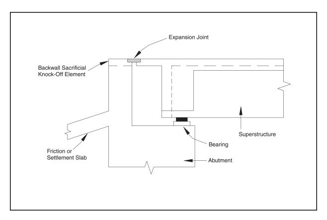
Figure 8-23. Knock-off device in backwall of seat-type abutment.
