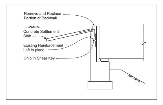
Figure 10-3. New Zealand style settlement slabs.
