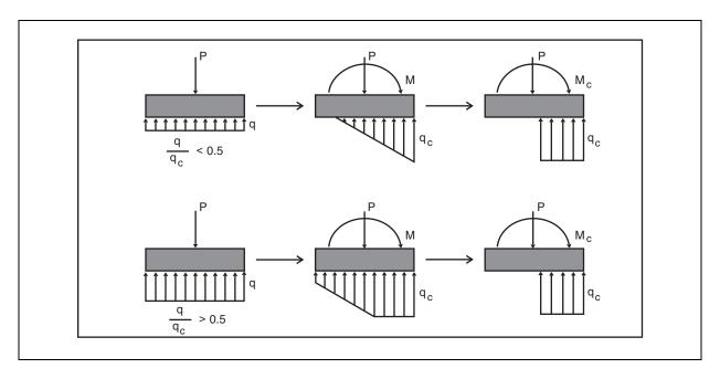
Figure 6-4. Idealized concentration of stress at edge of rigid footings subjected to overturning moment.
