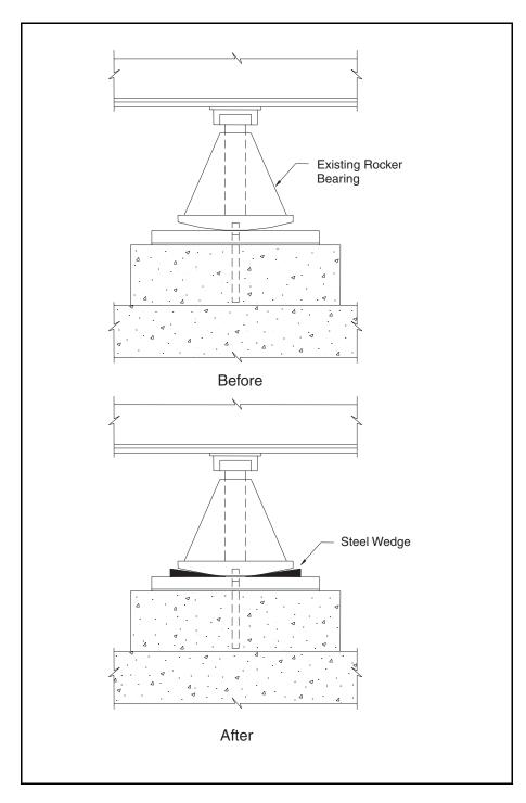
Figure 8-13. Expansion bearing retrofit.
