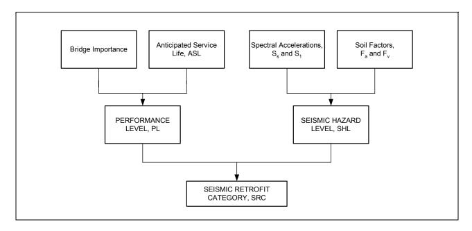
Figure 1-9. Determination of seismic retrofit category.
