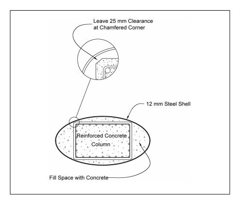
Figure 9-10. Typical steel shell retrofit of rectangular column.
