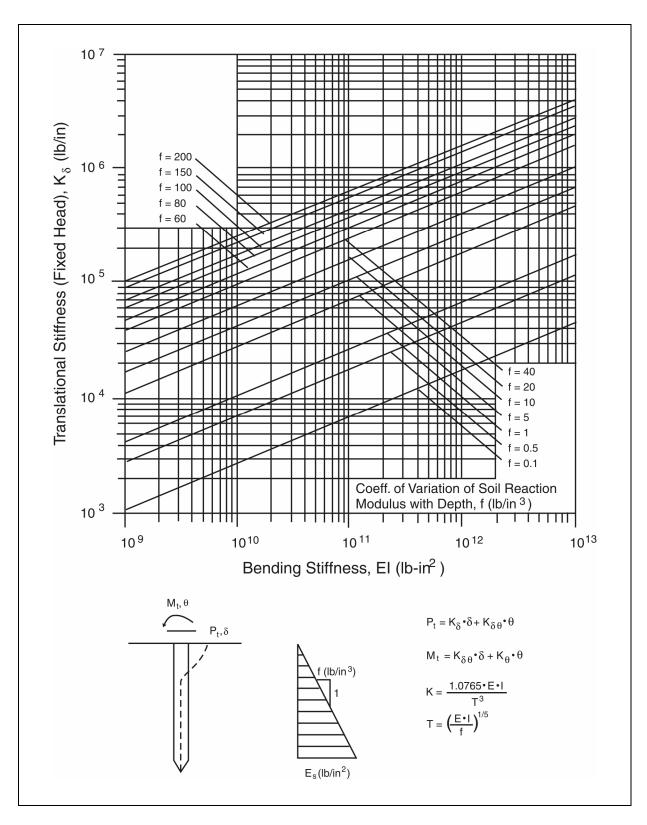
Figure 6-8. Lateral pile-head stiffness (fixed-head condition).
