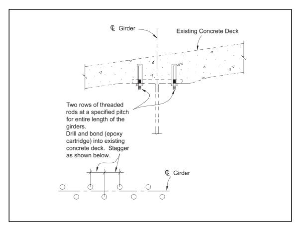
Figure 8-1. Deck to girder connection retrofit.
