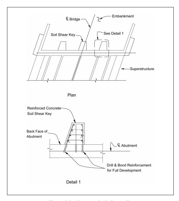
Figure 10-9. Abutment seismic shear walls.
