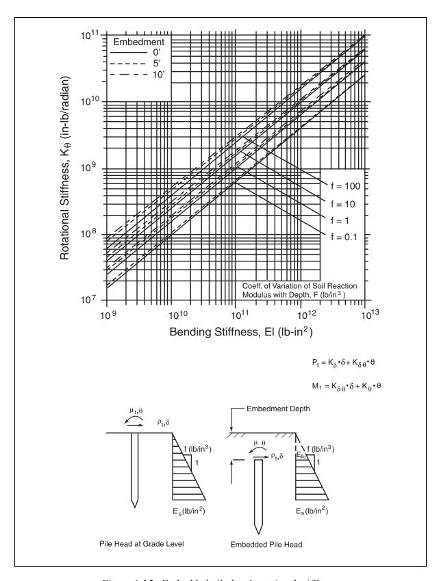
Figure 6-15. Embedded pile-head rotational stiffness.
