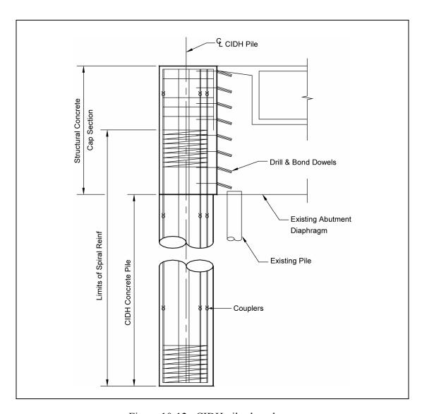
Figure 10-12. CIDH pile shear keys.
