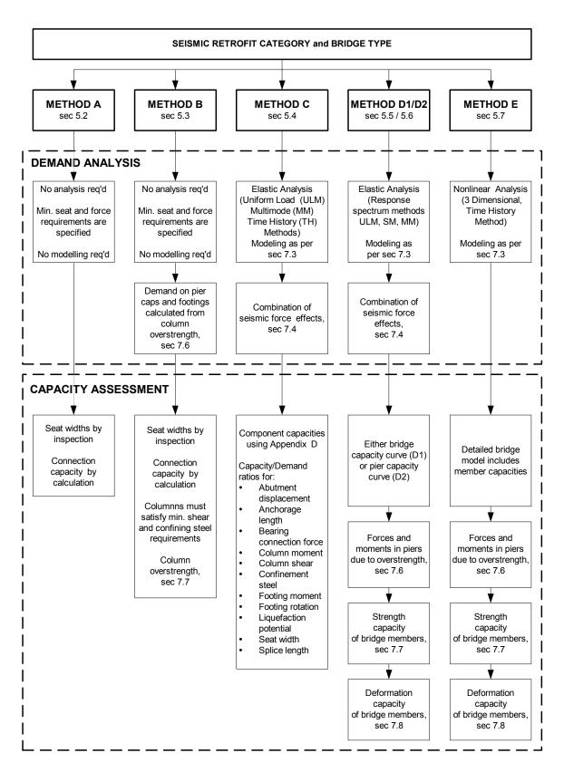
Figure 7-1. Evaluation methods for existing bridges showing relationship between demand analysis and capacity assessment.
