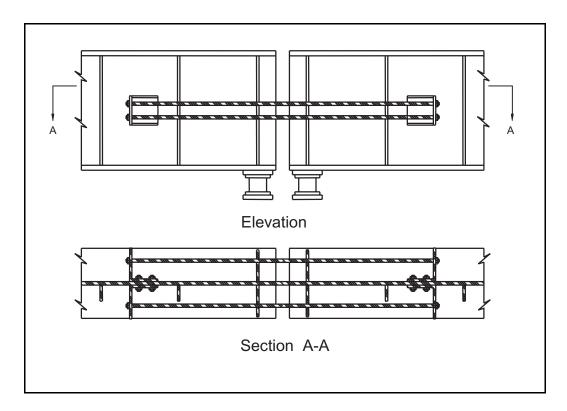
Figure 8-34. *Undesirable* restrainer detail.
