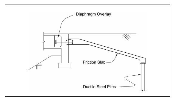
Figure 10-15. Modified abutment friction anchor.
