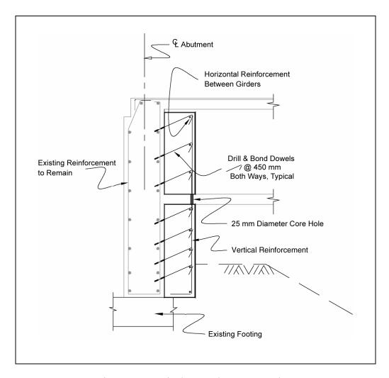
Figure 10-6. Diaphragm abutment overlay.
