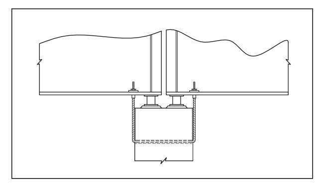
Figure 8-48. Vertical hold down retrofit.
