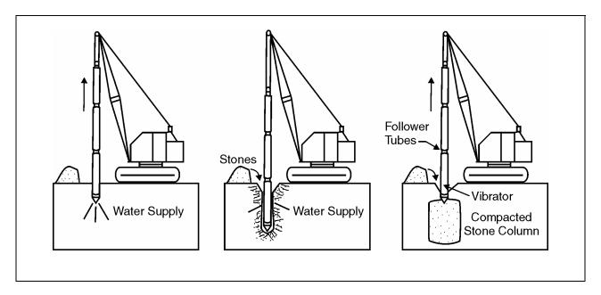
Figure 11-5. Vibro-replacement equipment and process.
