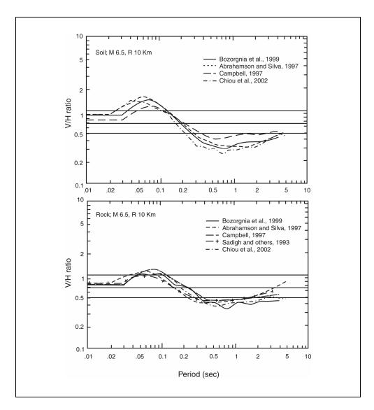
Figure 2-7. Vertical/horizontal spectral ratios vs. period
