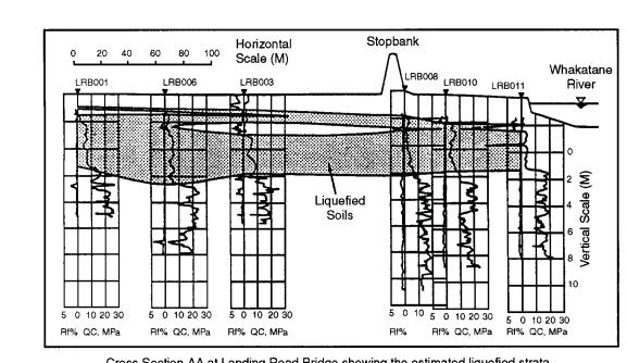
Cross Section AA at Landing Road Bridge showing the estimated liquefied strata Cross Section BB is generally similar, with the loose sand layer slightly thicker
