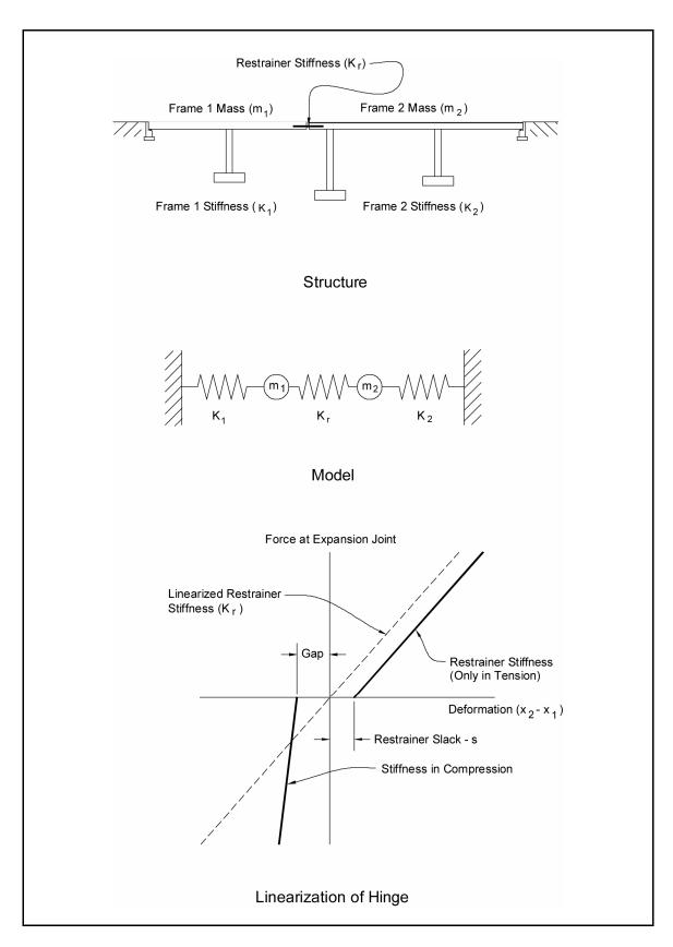
Figure 8-44. 2DOF model for the iterative method.
