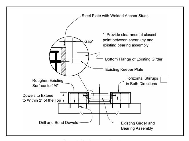
Figure 8-45. Transverse shear keys.
