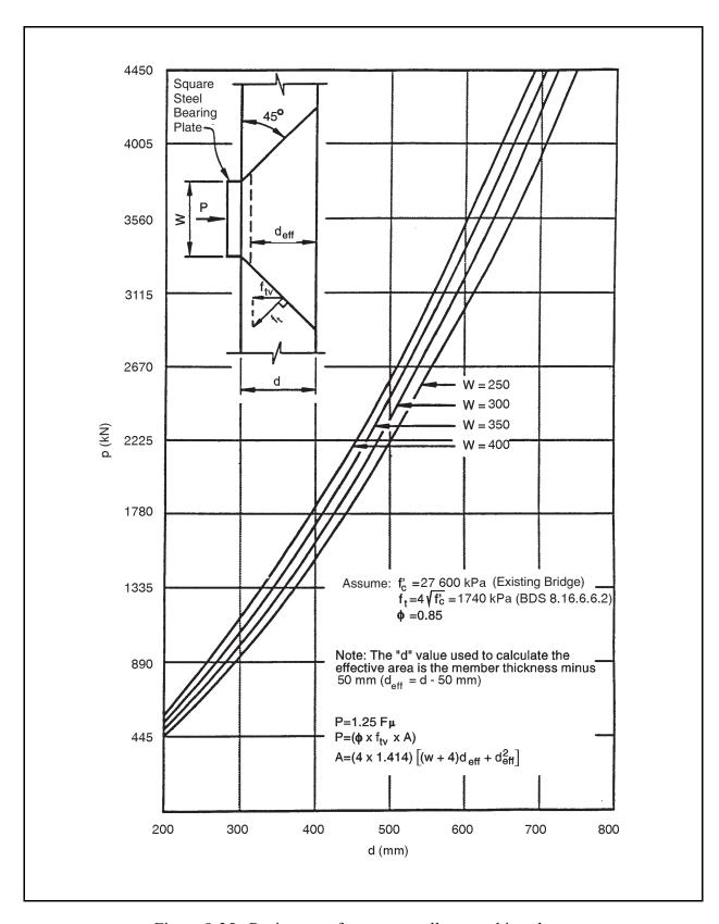
Figure 8-35. Resistance of concrete wall to punching shear.
