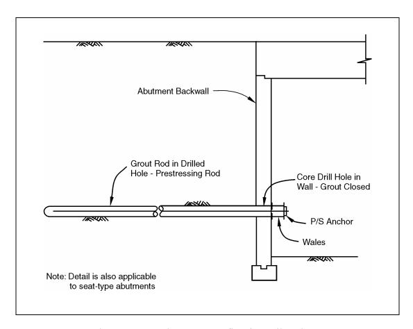
Figure 10-14. Abutment retrofit using soil anchors.
