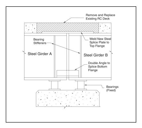
Figure 8-8. Girders made continuous for live load.
