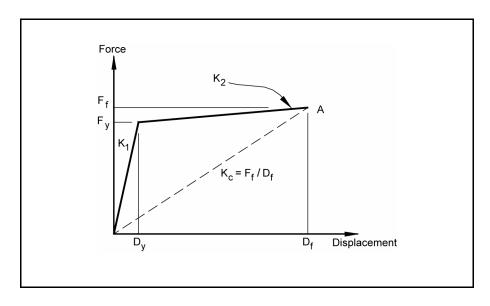
Figure 8-43. Force displacement relationship for abutment.
