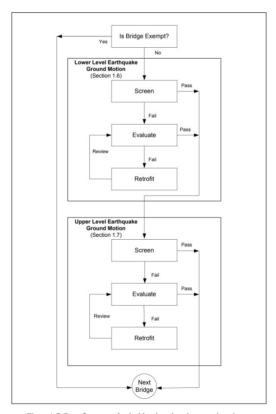
Figure 1-7. Retrofit process for dual level earthquake ground motions.
