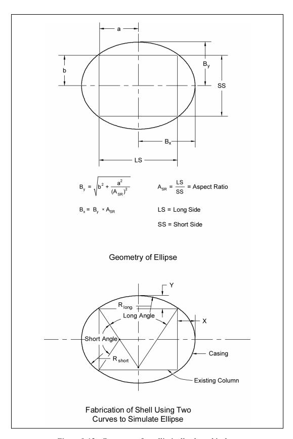
Figure 9-12. Geometry of an elliptically shaped jacket.
