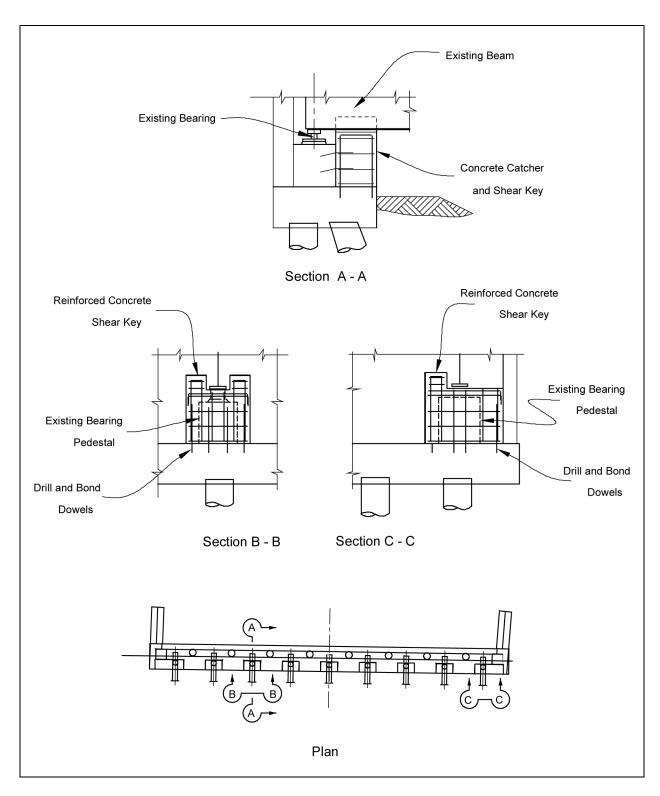
Figure 10-7. Concrete block abutment shear key.
