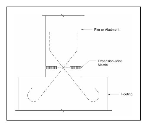
Figure 8-24. Freyssinet hinge.
