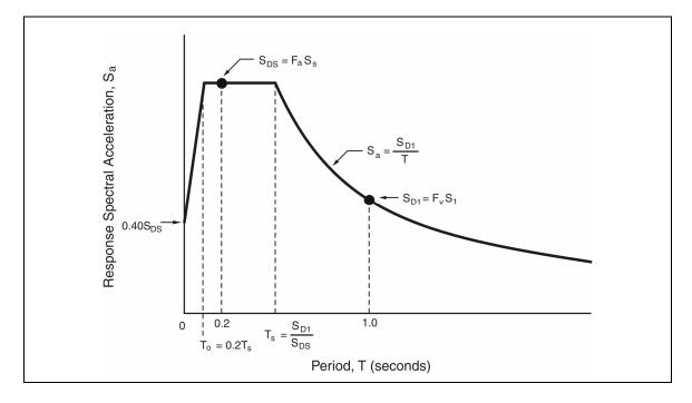
Figure 1-8. Construction of the seismic design response spectrum.
