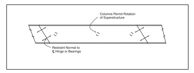
Figure 8-37. Restrainer orientation for transversely flexible supports.
