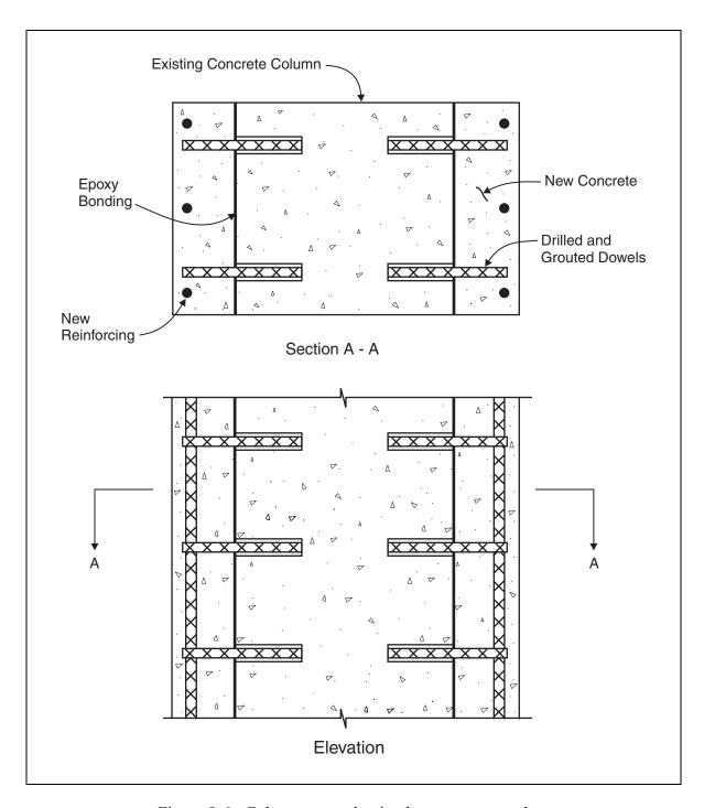
Figure 9-6. Column strengthening by concrete overlay.
