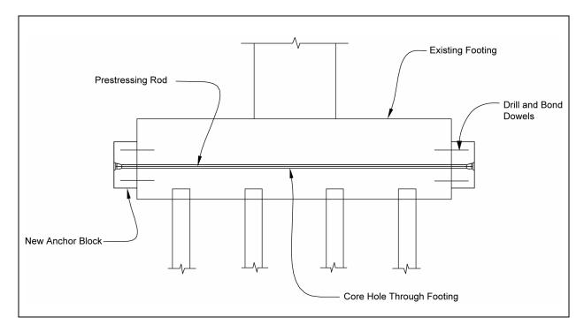
Figure 10-19. Footing strengthening by horizontal prestressing.
