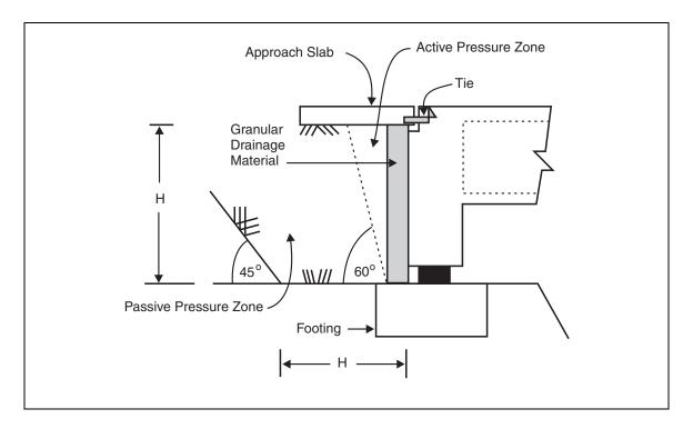
Figure 6-23. Design passive pressure zone.
