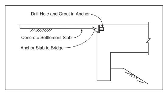
Figure 10-2. California style settlement slabs.
