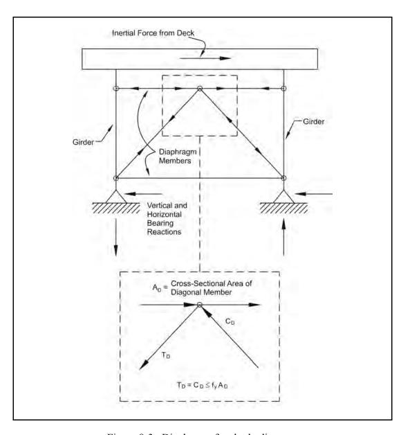
Figure 8-3. Diaphragm free body diagram.
