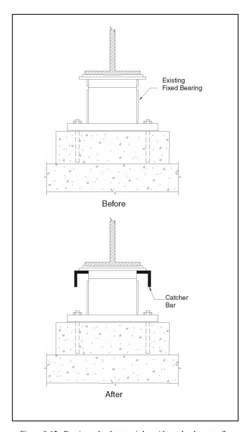
Figure 8-12. Bearing sole plate to girder with catcher bar retrofit.
