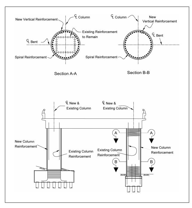
Figure 9-2. Column replacement using existing column reinforcement.
