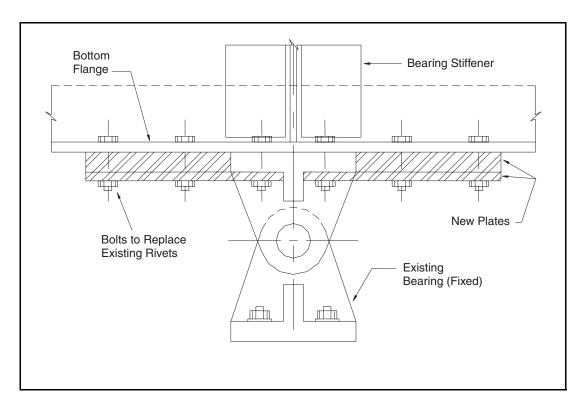
Figure 8-11. Bearing sole plate to girder connection retrofit.
