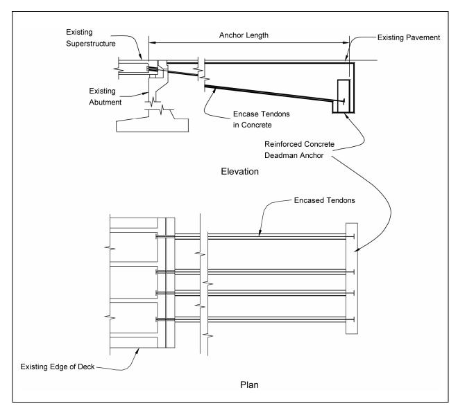
Figure 10-13. Gravity or "Deadman" anchors.
