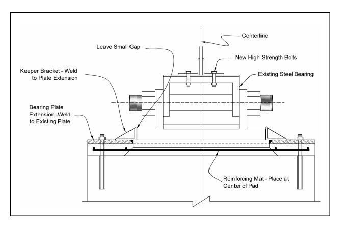
Figure 8-46. Bearing keeper bracket retrofit.
