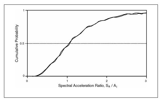
Figure C-2. A normalized fragility curve based on a lognormal probability distribution with a coefficient of dispersion  $\beta_c = 0.6$ .
