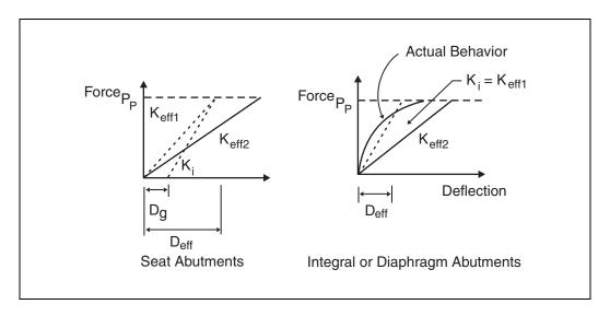
Figure 6-24. Characterization of abutment capacity and stiffness.
