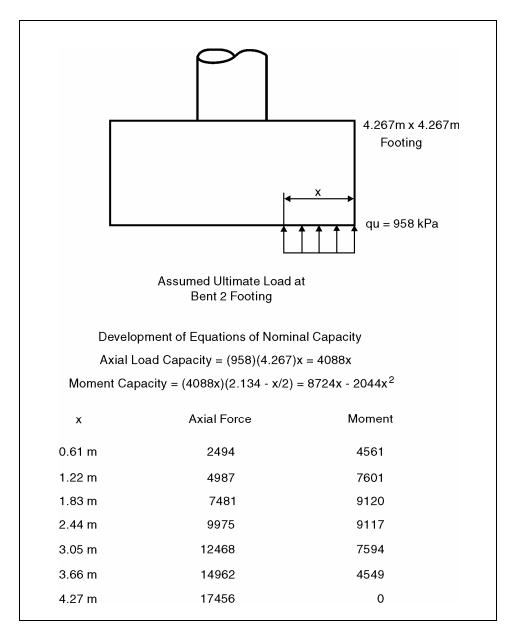
Figure E-8. Development of footing interaction diagram at bent 2.
