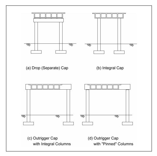
Figure 9-27. Typical cap beam configurations for boxgirder bridges.
