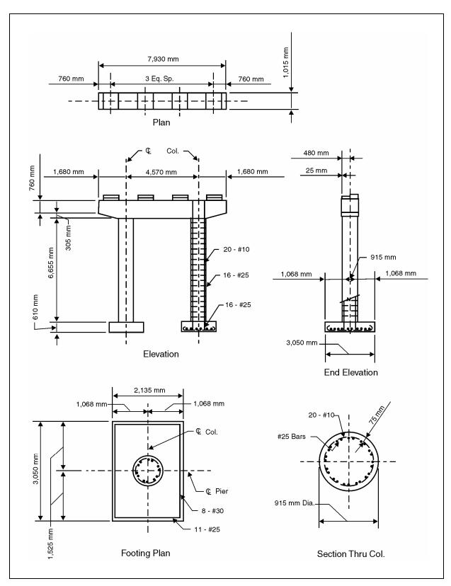
Figure F-2. Pier 2 bent details.
