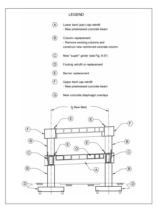
Figure 9-1. Column replacement on San Francisco viaducts.
