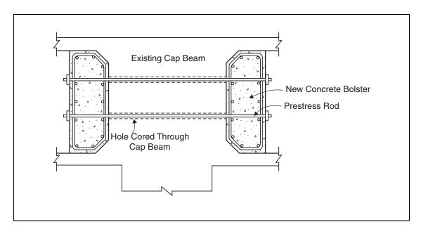
Figure 9-36. Retrofit of an integral cap beam joint for longitudinal loading.
