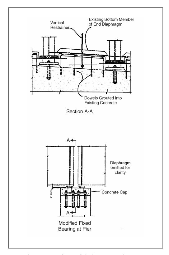
Figure 8-17. Bearing retrofitting by encasement in concrete.
