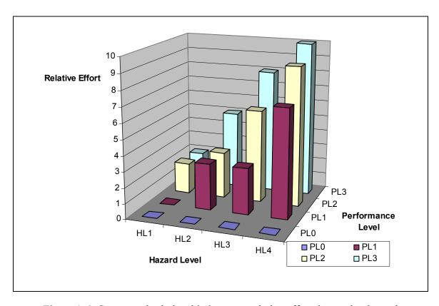
Figure 1-6. Conceptual relationship between relative effort, increasing hazard and performance criteria implied in this manual.
