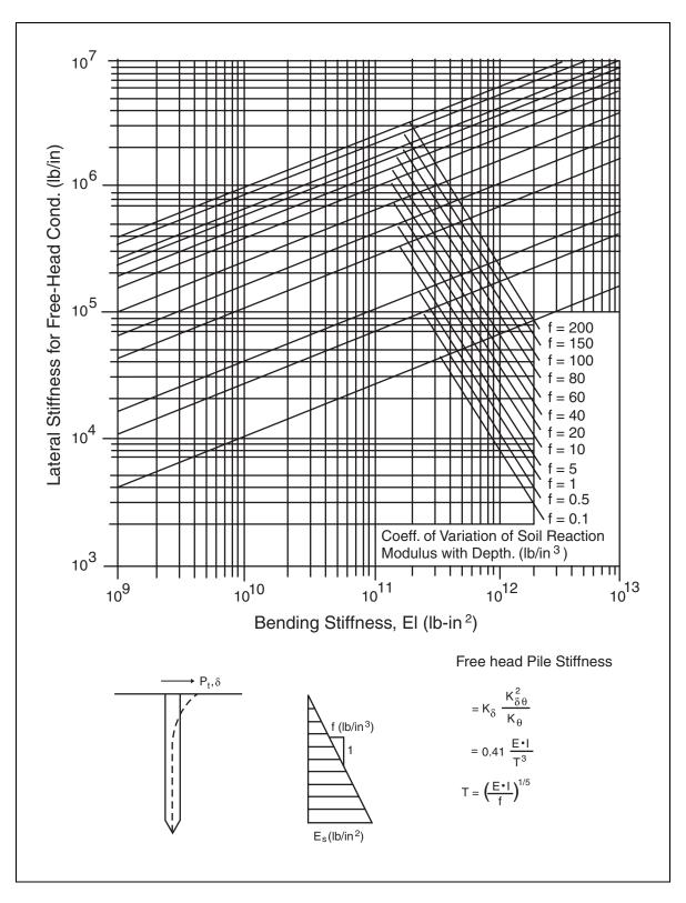
Figure 6-11. Lateral pile-head stiffness (free-head condition).
