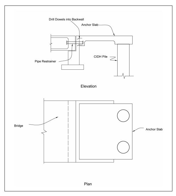
Figure 10-5. Anchor slabs with CIDH piles.
