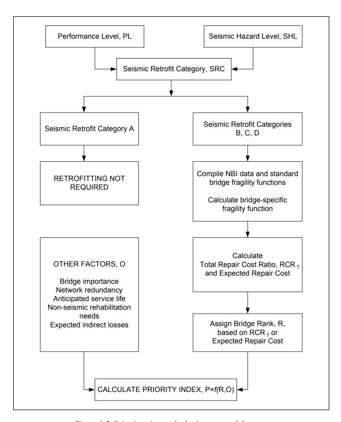
Figure 4-5. Seismic rating method using expected damage.
