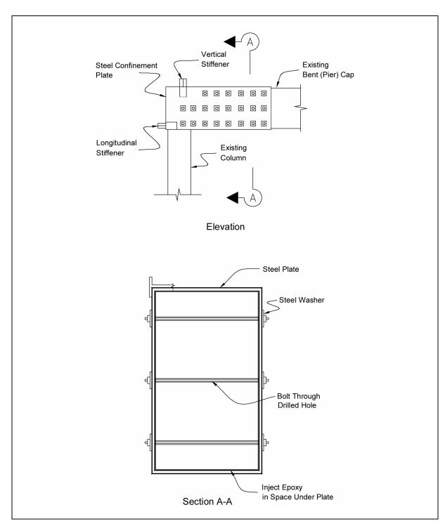
Figure 9-35. Knee joint retrofit with steel plates.
