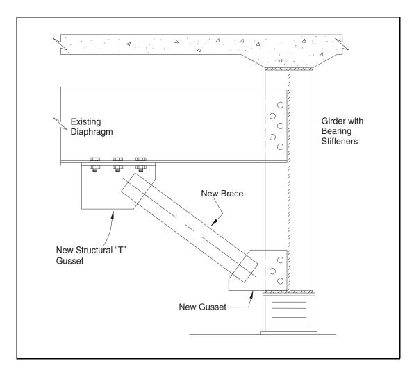
Figure 8-5. Girder bracing retrofit.
