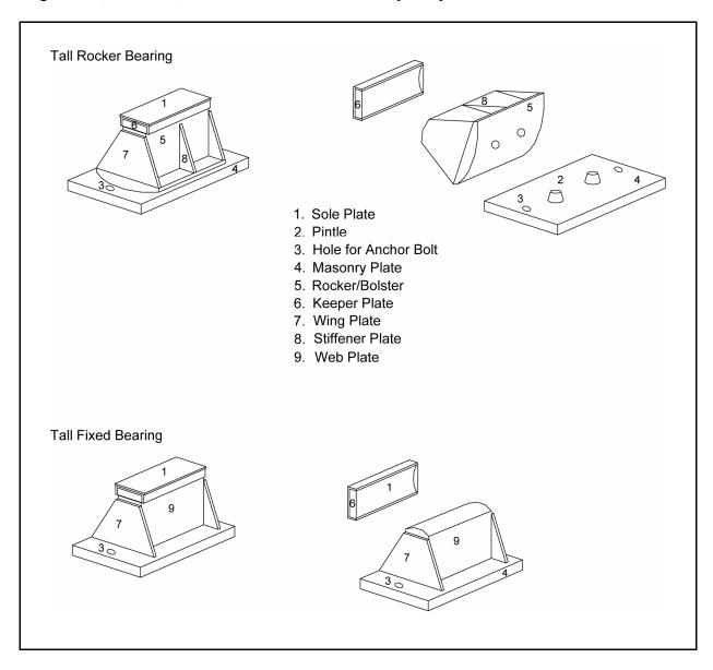
Figure 8-10. Steel bearing nomenclature.
