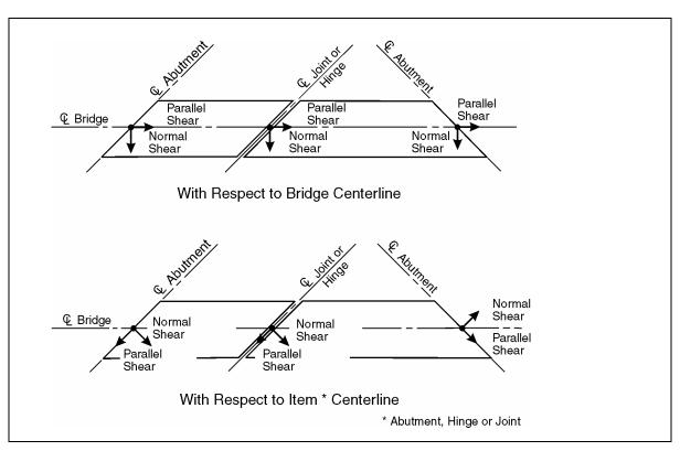
Figure E-4. Positive sign convention for abutment, hinge and joint forces.
