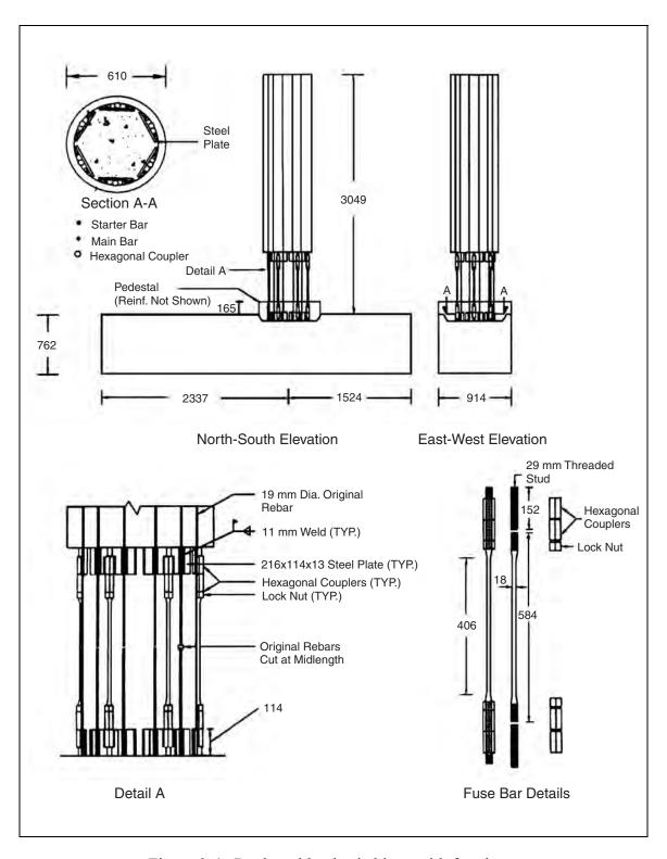
Figure 9-4. Replaceable plastic hinge with fuse bars.
