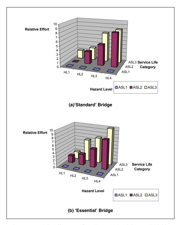
Figure 1-11. Relative effort to retrofit an (a) 'standard' and (b) 'essential' bridge with varying service life and hazard level.
