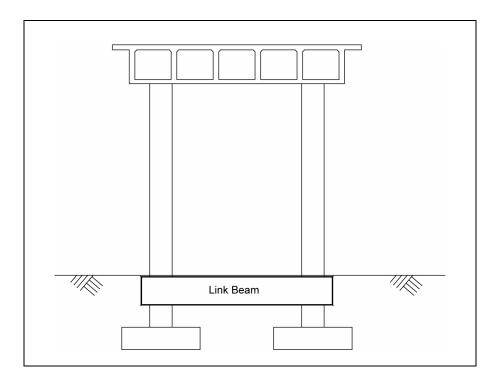
Figure 10-24. Footing link beam retrofit.
