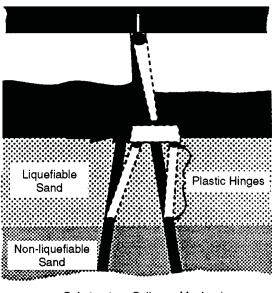
Substructure Collapse Mechanism
