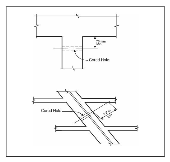
Figure 8-39. Required clearances for coring.
