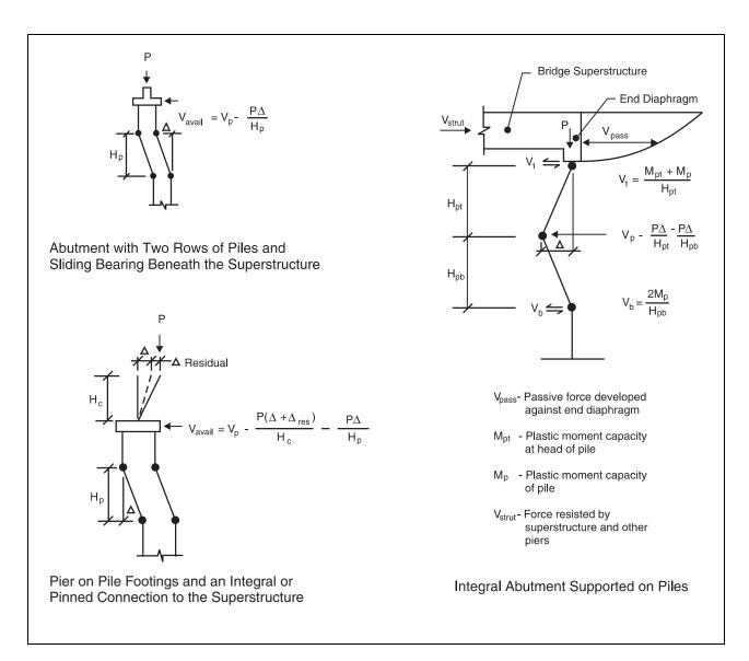
Figure 11-4. Corrections for P- $\Delta$  effects in piles with plastic hinges.
