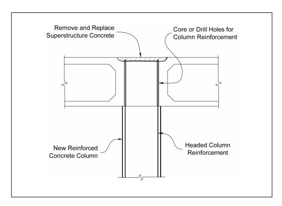
Figure 9-3. Column anchorage using headed reinforcement.
