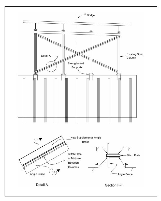
Figure 9-22. Retrofit of X-braced steel bent.
