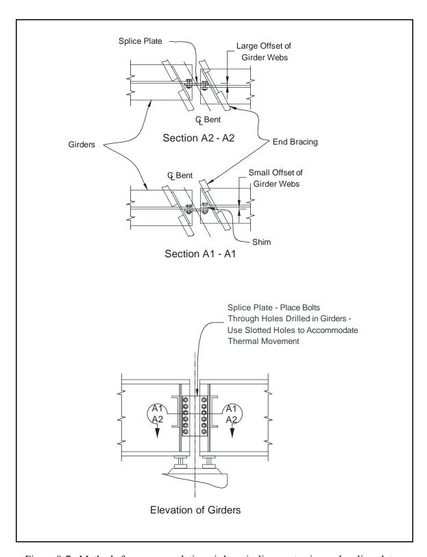
Figure 8-7. Methods for accommodating girder misalignment using web splice plates.
