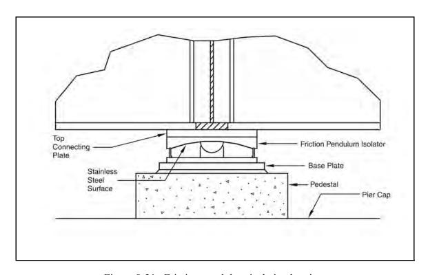
Figure 8-21. Friction-pendulum isolation bearing.
