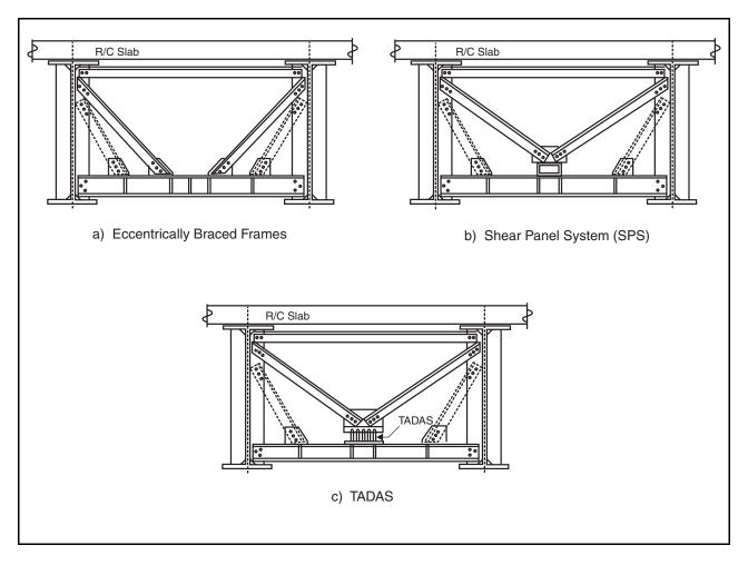
Figure 8-4. Ductile end diaphragms.
