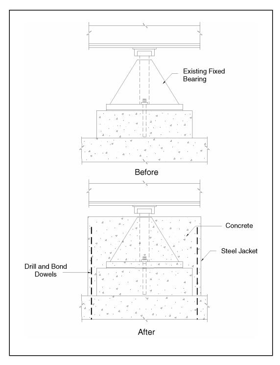
Figure 8-16. Bearing retrofitting by encasement in steel shell.
