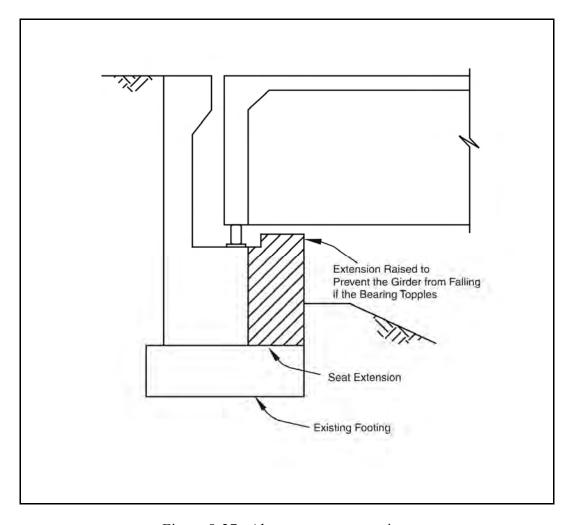
Figure 8-27. Abutment seat extension.
