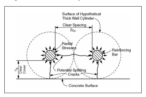
Figure D-7. Radial stresses developed due to bar anchorage.
