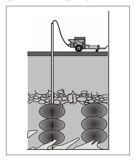
Figure 11-8. Compaction grout bulb construction.
