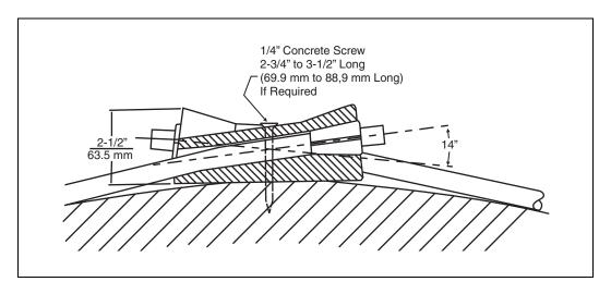
Figure 9-14. Anchorages for prestress strand retrofit.
