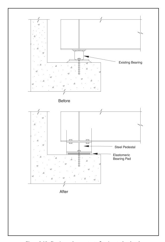
Figure 8-18. Bearing replacement retrofit using steel pedestal.
