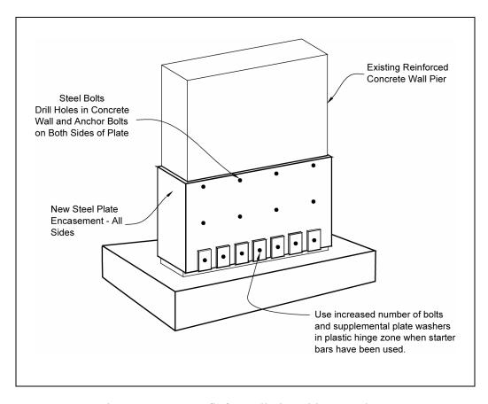
Figure 9-26. Retrofit for wall pier with starter bars.
