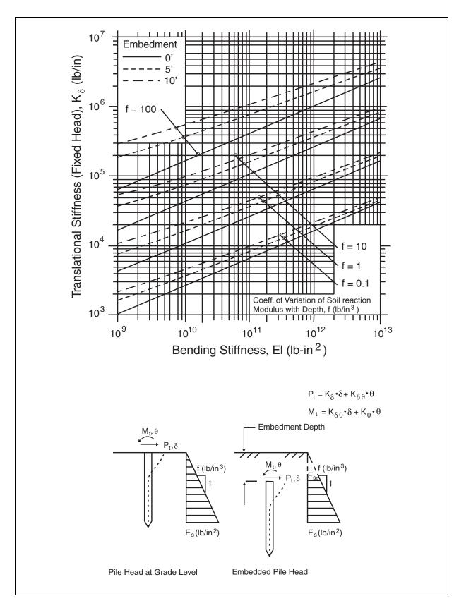
Figure 6-14. Lateral embedded pile-head stiffness (fixed-head condition).
