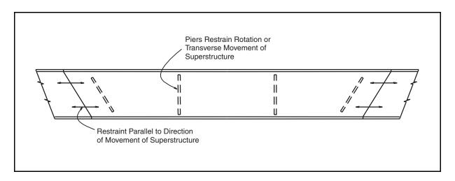
Figure 8-36. Restrainer orientation for transversely rigid supports.
