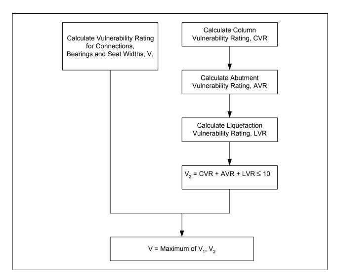
Figure 4-2. Calculation of bridge vulnerability, V.
