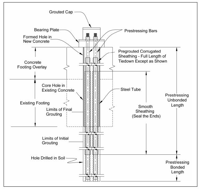
Figure 10-25. Prestressed tie-down anchor.
