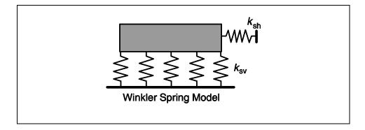
Figure 6-2. Uncoupled Winkler spring model.
