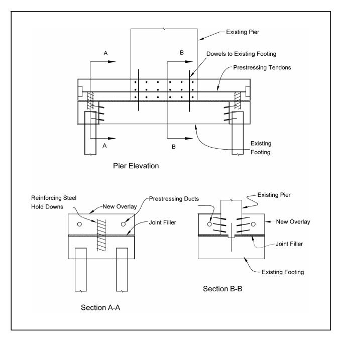
Figure 8-26. Concrete hinge retrofit
