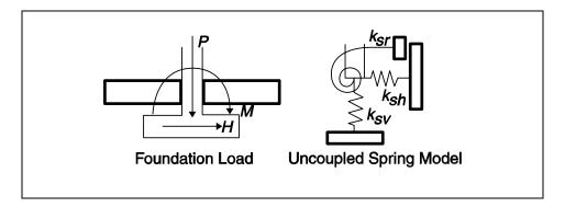
Figure 6-1. Uncoupled elasto-plastic spring model for rigid footings.
