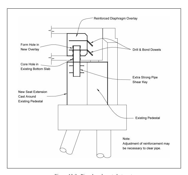
Figure 10-8. Pipe shear key at abutment.
