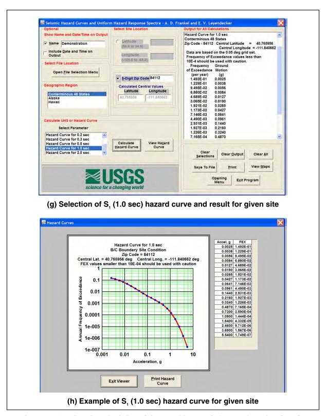
Figure 2-3 (continued). Calculation of short- and long-period spectral accelerations for 100- and 1000-year ground motion return periods.
