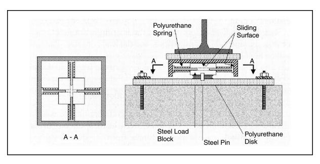
Figure 8-22. Eradiquake isolation bearing.
