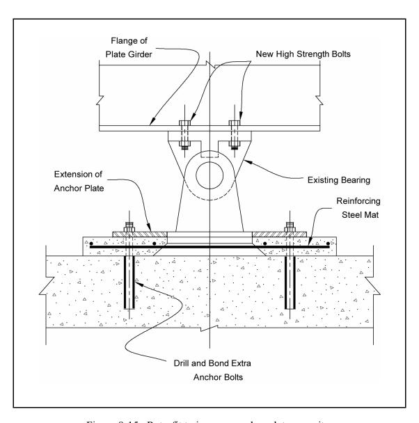
Figure 8-15. Retrofit to increase anchor plate capacity.
