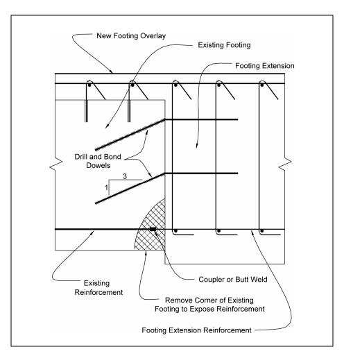
Figure 10-18. Bottom reinforcing splice detail.
