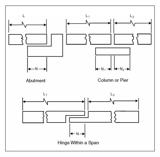
Figure D-1. Minimum support length requirements.
