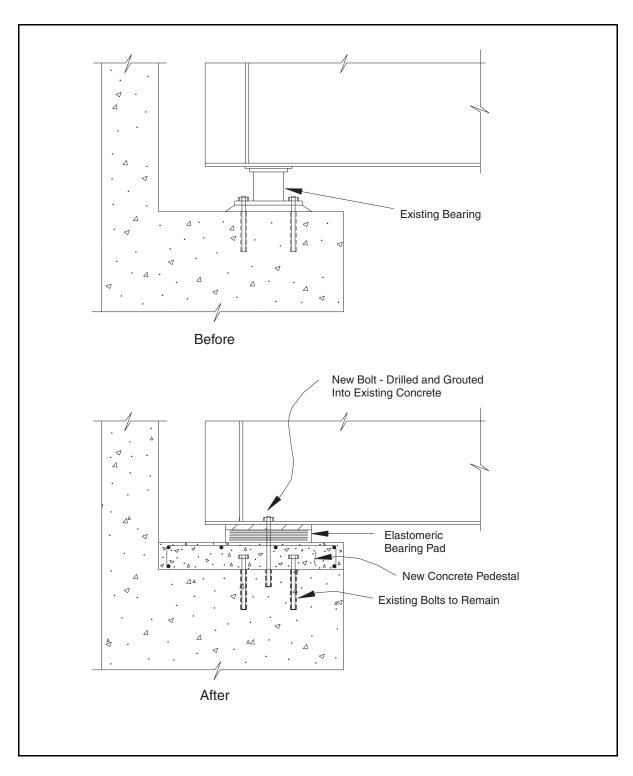
Figure 8-19. Bearing replacement using concrete pedestal.
