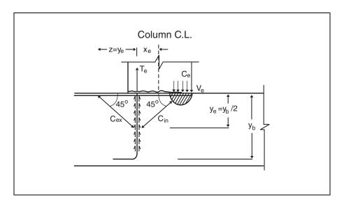
Figure 10-22. Strut and tie model for joint design.
