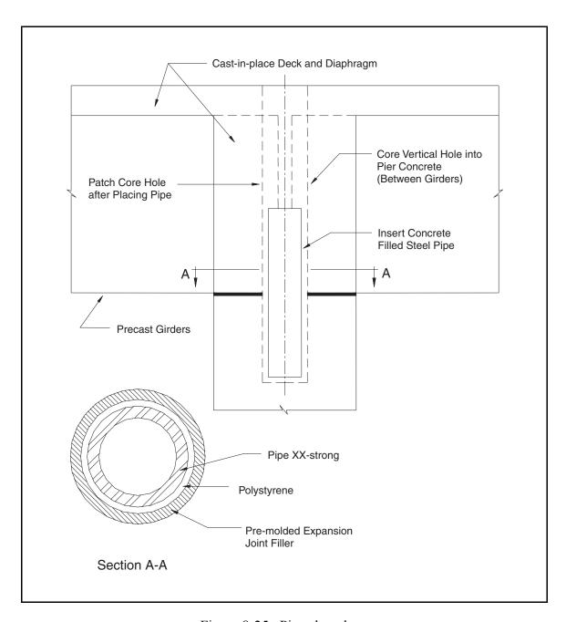
Figure 8-25. Pipe shear key.
