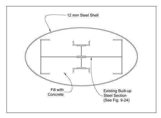
Figure 9-25. Built-up steel column retrofitted with steel shell.
