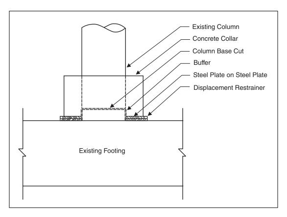
Figure 9-21. Column retrofit by flexural strength reduction.
