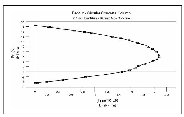
Figure F-3. Column interaction diagram.
