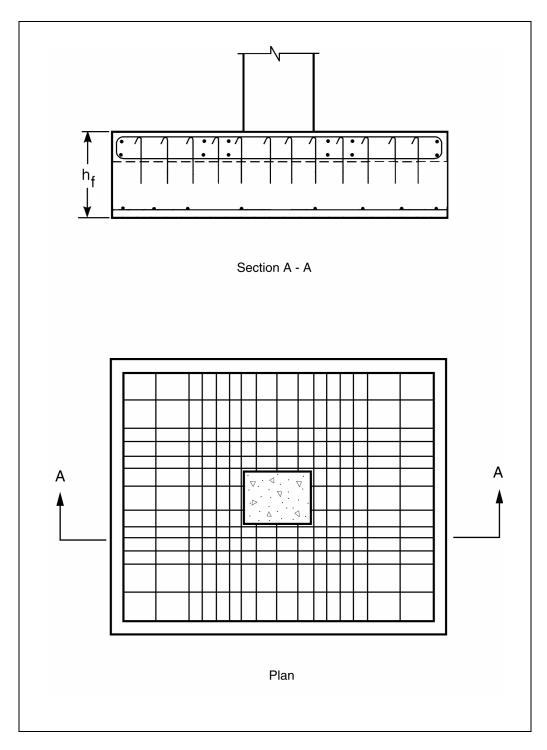
Figure 10-17. Footing retrofit with concrete overlay.
