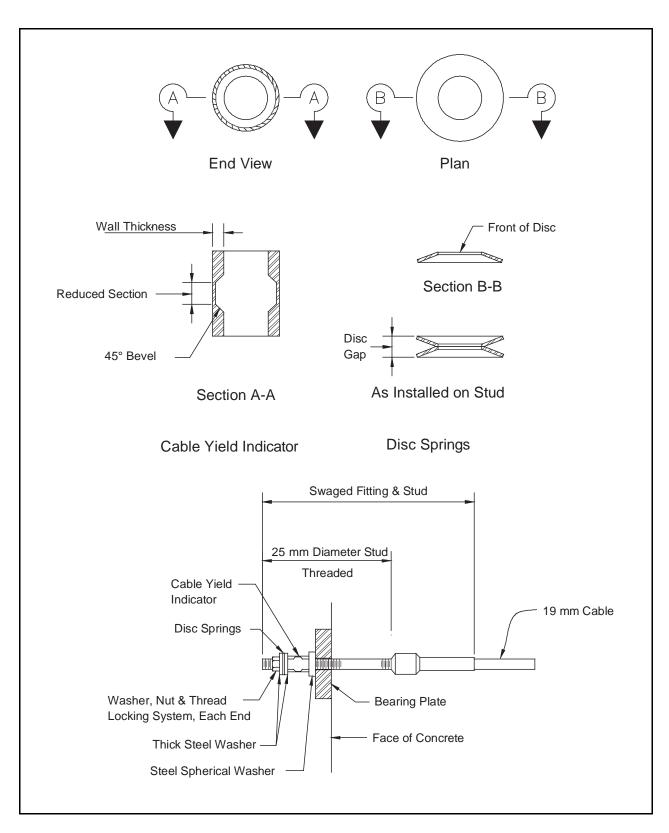
Figure 8-29. Caltrans cable restrainer unit.
