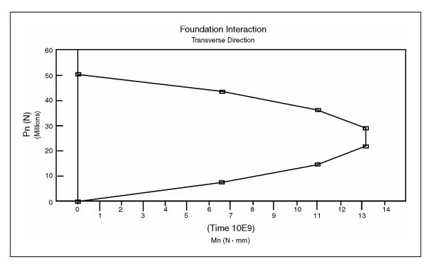
Figure F-5. Foundation interaction diagram - transverse direction.
