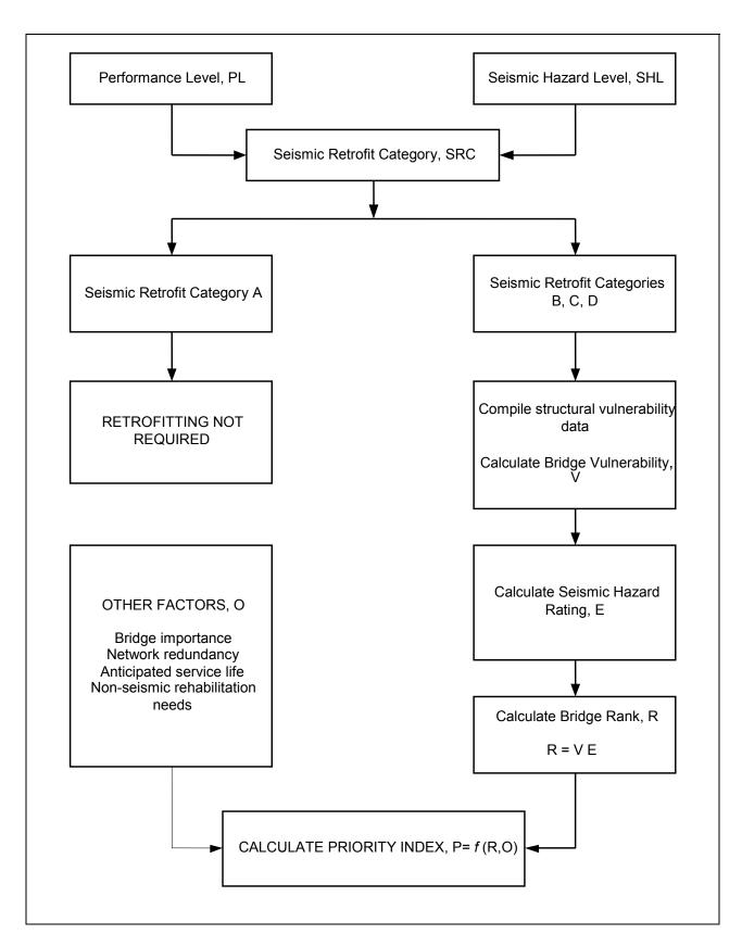
Figure 4-1. Seismic rating method using indices.
