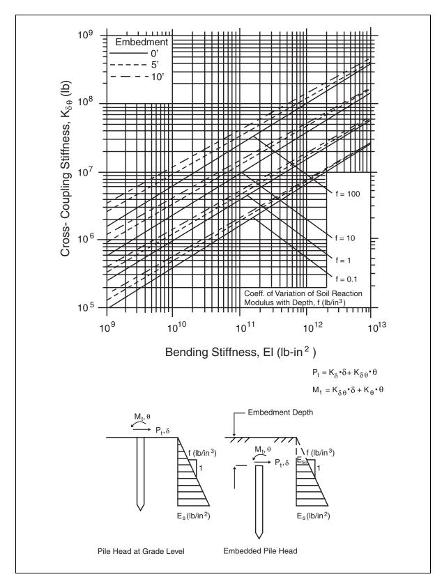
Figure 6-16. Embedded pile cross-coupling pile-head stiffness.
