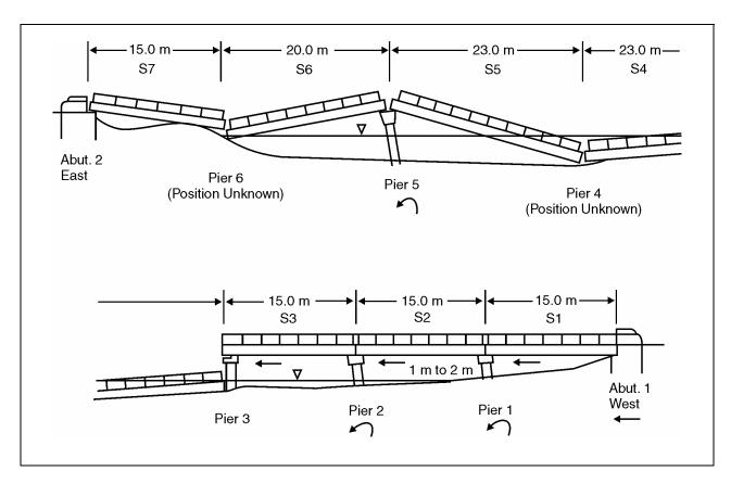
Figure 6-26. Sketch of Magsaysay bridge showing earthquake damage.
