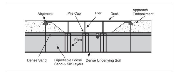
Figure 11-1. Elevation view of a representative bridge on a liquefiable stratum.
