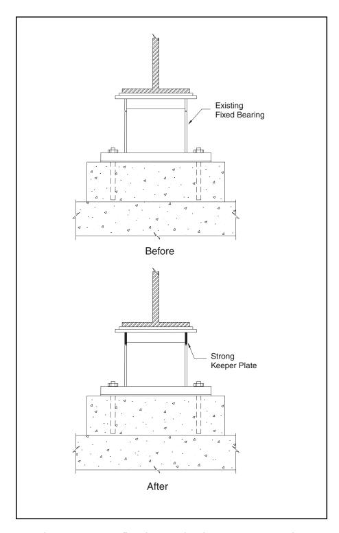
Figure 8-14. Retrofit to increase bearing transverse capacity.
