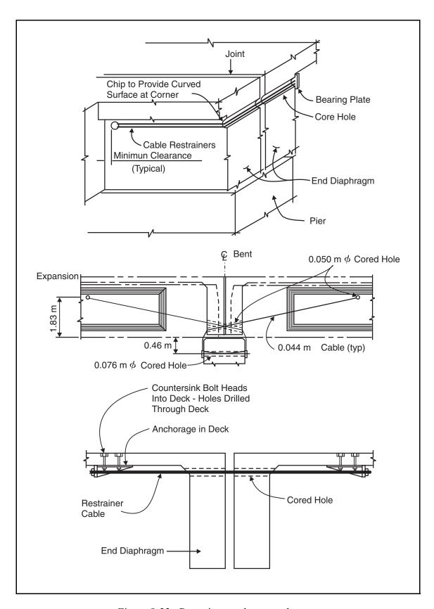
Figure 8-33. Restrainer anchorage schemes.
