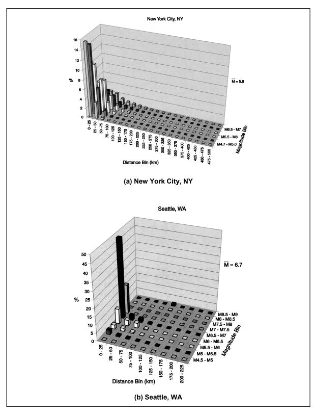
Figure 2-8. Hazard deaggregation for 0.2 second response spectral acceleration ( $S_s$ ) for ground motion with three percent probability of exceedance in 75 years (2500-year return period).
