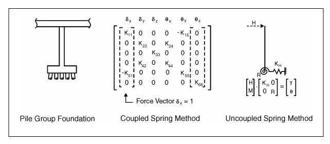
Figure 6-18. Modeling approaches for deep foundations.
