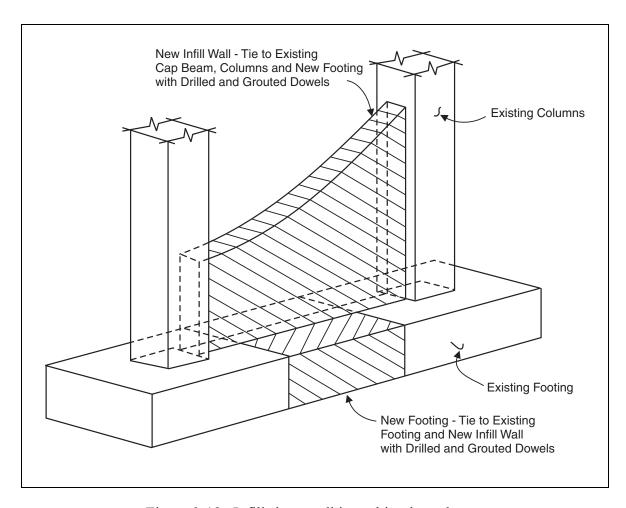
Figure 9-18. Infill shear wall in multi-column bents.
