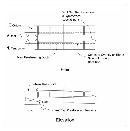
Figure 9-28. Pier cap strengthening.
