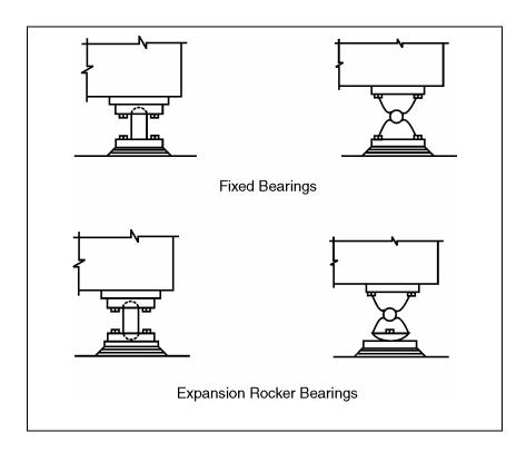
Figure 4-3. Seismically vulnerable bearings.
