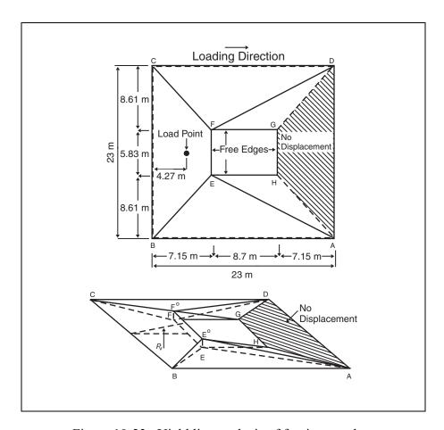
Figure 10-23. Yield line analysis of footing overlay.
