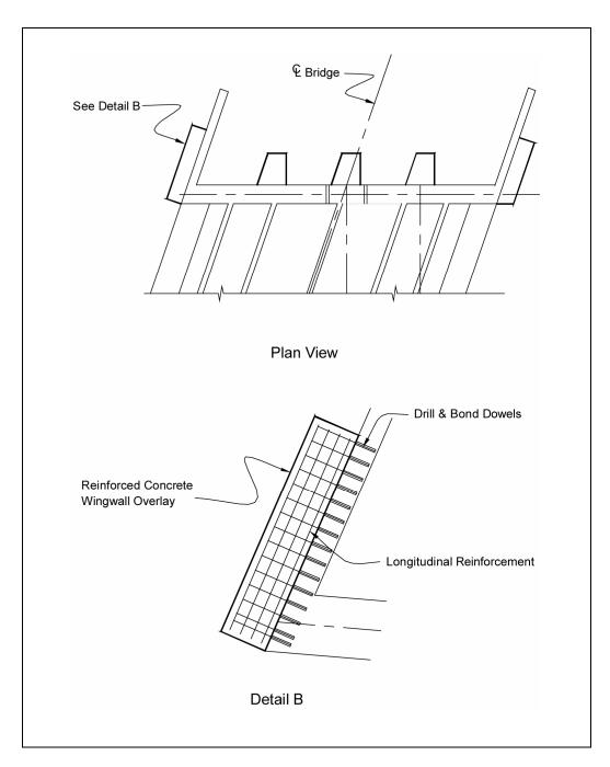
Figure 10-10. Wingwall overlay.
