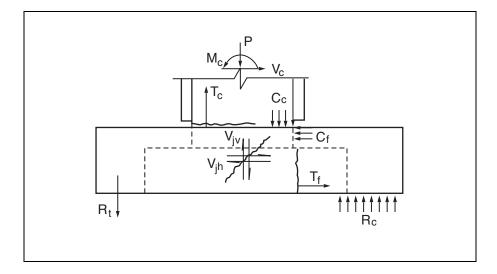
Figure 10-21. Footing joint shear forces.
