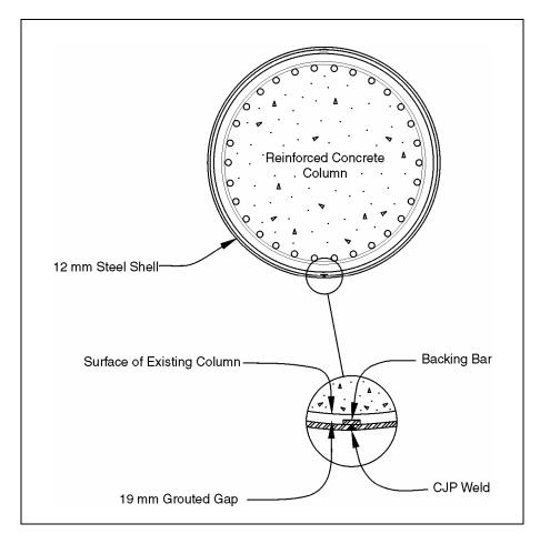
Figure 9-9. Typical steel shell retrofit of round column.
