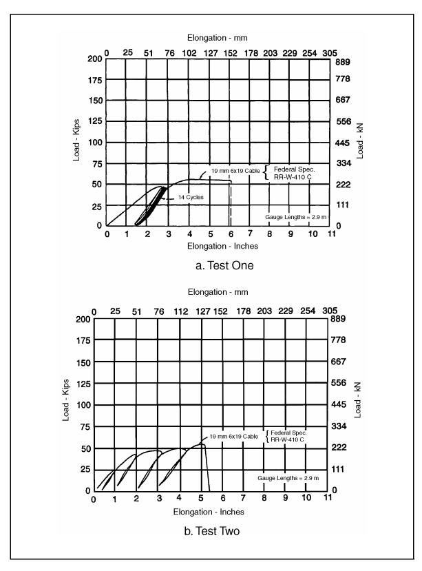
Figure 8-30. Caltrans tests of restrainer cable.
