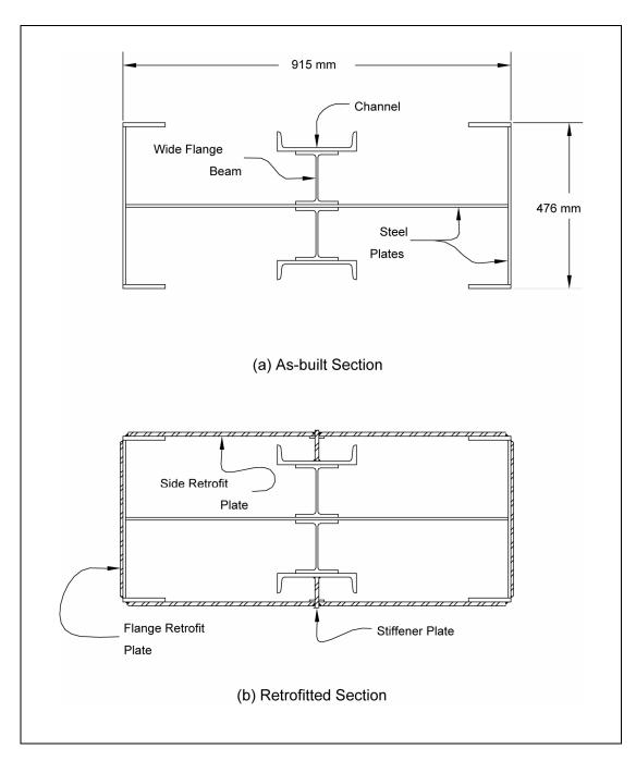
Figure 9-24. Built-up steel columns stiffened by plates.
