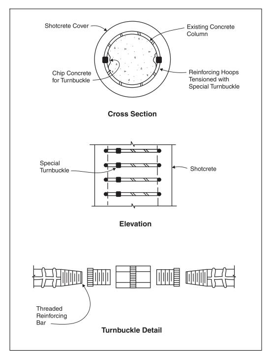
Figure 9-16. Semi-circular reinforcing bars with couplers.
