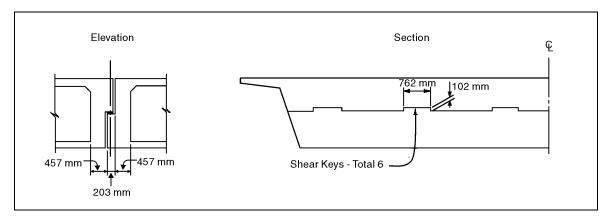
Figure E-2. Expansion joint detail.
