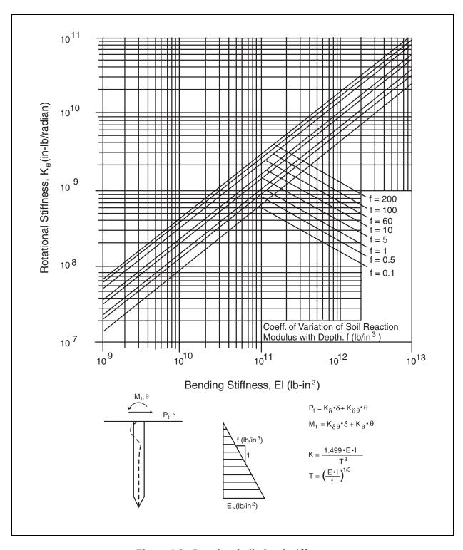
Figure 6-9. Rotational pile-head stiffness.
