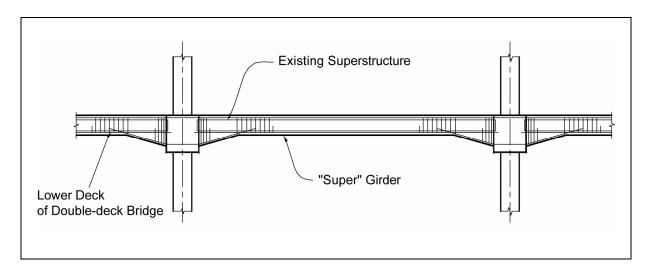
Figure 9-37. "Supergirders" added between piers to reduce torsion in pier caps.
