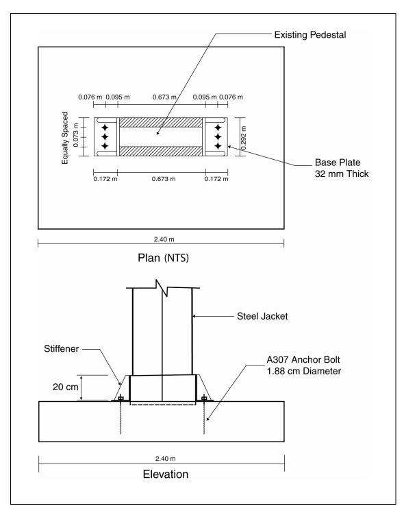
Figure 9-8. Column strengthening by anchoring steel shell.
