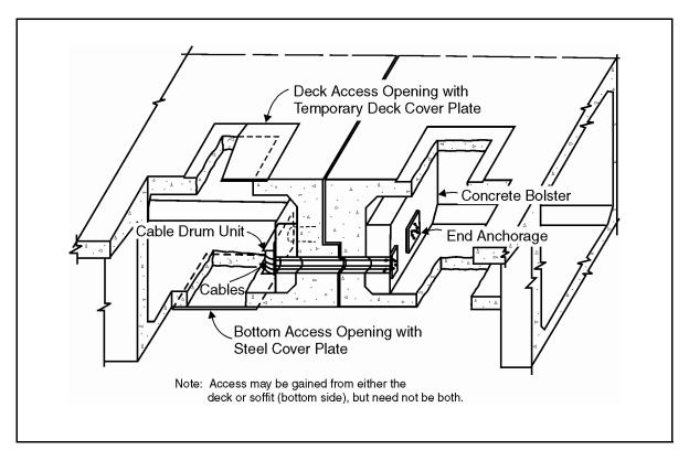
Figure 8-31. Multi-cable restrainer assembly.
