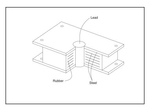
Figure 8-20. Lead-filled elastomeric isolation bearing.
