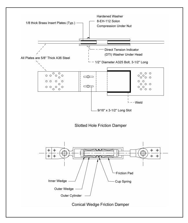
Figure 8-50. Friction dampers.
