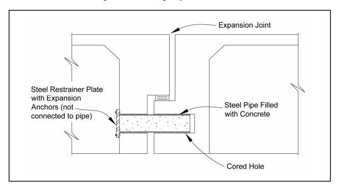
Figure 8-47. Steel pipe restrainers.
