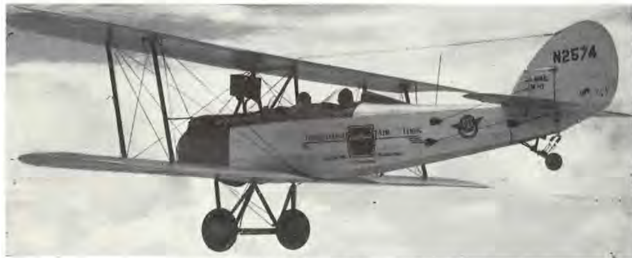
Figure 1. 1927 OX-5 powered Waco 9 — 80-mph mail plane operated by Pennsylvania Airlines. Note extra wing, propeller, interplane struts, "streamlined" wires, radiator, landing gear and tail wheel amounting to a built-in "head-wind." Due to the "design drag," cleanliness had little effect on speed.
