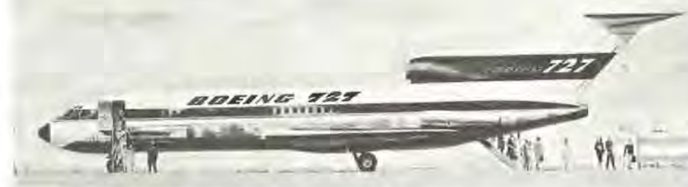
FIG. 1 —Short ground times will be a feature of the 727 to enable operators to offer fast service on routes with many short segments. An air-stair at the rear will be basic on 727s. A forward entry may be provided with a similar air-stair as an optional feature.
