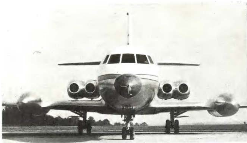
Figure 5. Lockheed JetStar. 8-10 passenger 500 MPH business aircraft ordered by several corporations. The four tail mounted turbojets are 3000 lb. thrust P & W JT-12's. The wing "glove" tanks each hold 640 gallons of kerosene. Predicted range 2900 miles.
