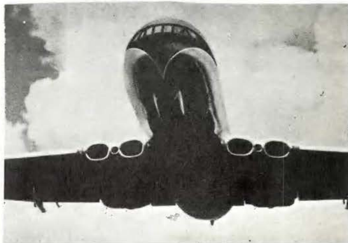
Figure 6. English de Havilland Comet 4B 72 passenger 450 MPH 3000 mile range aircraft operated by BOAC to feed their big American jets. Four 10,500 lb. thrust Rolls Royce Avon Turbojets "imbedded" in the wings. The Comet I accidents of 1952-1954 era provided designers considerable information regarding jet aircraft safe design requirements. Engine serviceability unsatisfactory to most designers.
