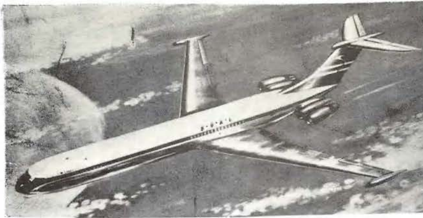
Figure 8. English Vickers VC-10, 575 MPH, 200 passenger aircraft, slated for BOAC transocean competition with big U.S. jets about 1965. Unlike the above DH121 which is about to be flown, this is an artist's conception. Some components are under construction.
