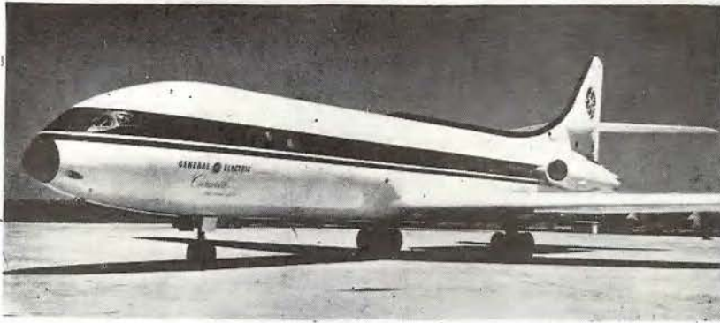
Figure 3. French Caravelle 530 MPH, 60-80 passenger, 6700 ft. runway (60° F day) upto 1500 mile range aircraft bought by United Airlines. Two Rolls Royce Avon engines, one mounted each side of rear end of fuselage. (Passenger tail loading ramp like Martin 404.)
