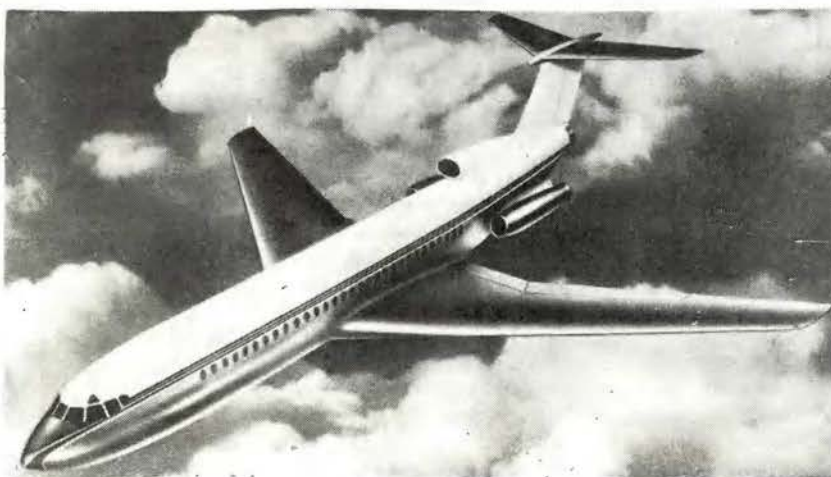
Figure 7. English Triple turbojet (the RR Avon 10,500 lb. thrust) Turbojet engines mounted in the rear fuselage of the de Havilland 121, 100 passenger 600 MPH, short haul (up to 1700 miles), 7000 ft. runway feeder aircraft. Eastern Airlines said to be dickering with Boeing for similar triple turbojet Model 727 with Allison built Rolls Royce engines.
