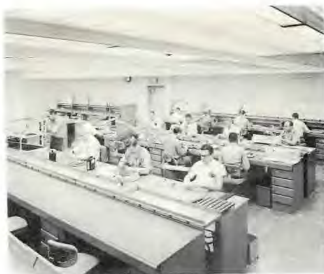
Here is where one-of-a-kind prototypes and other special projects for flight inspection aircraft come into being. Component boards, cables, control boxes, consoles, racks, and other special items are fabricated and wired in this shop.
