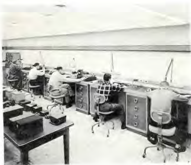
This shop repairs and calibrates all electrical meters and indicators used in airborne electronic equipment aboard flight inspection aircraft. Transfer standards on the work benches are calibrated weekly against primary standards which, in turn, are calibrated by the Bureau of Standards every year.
