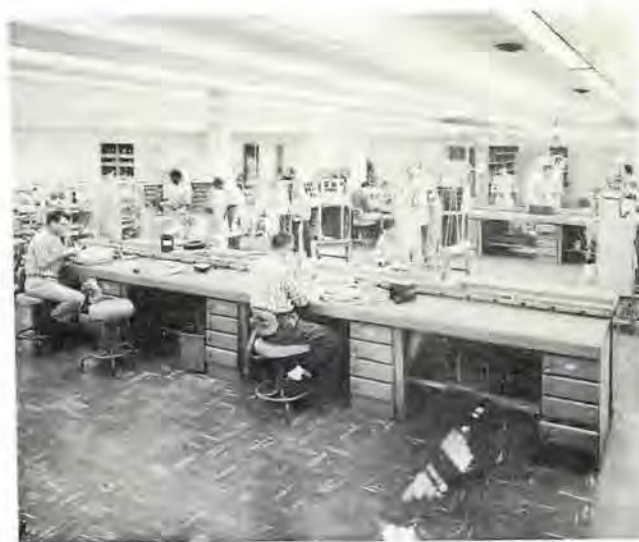
This is the shop that produces the specialized equipment used in the electronic systems aboard flight inspection aircraft. FAA and military flight inspection aircraft being modified to a standardized configuration have their electronic equipment built and installed by technicians from this shop.
