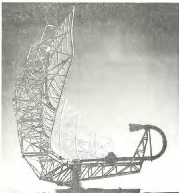
The antenna of the long-range radar which "transmits" and "receives" the radar target pulse.
