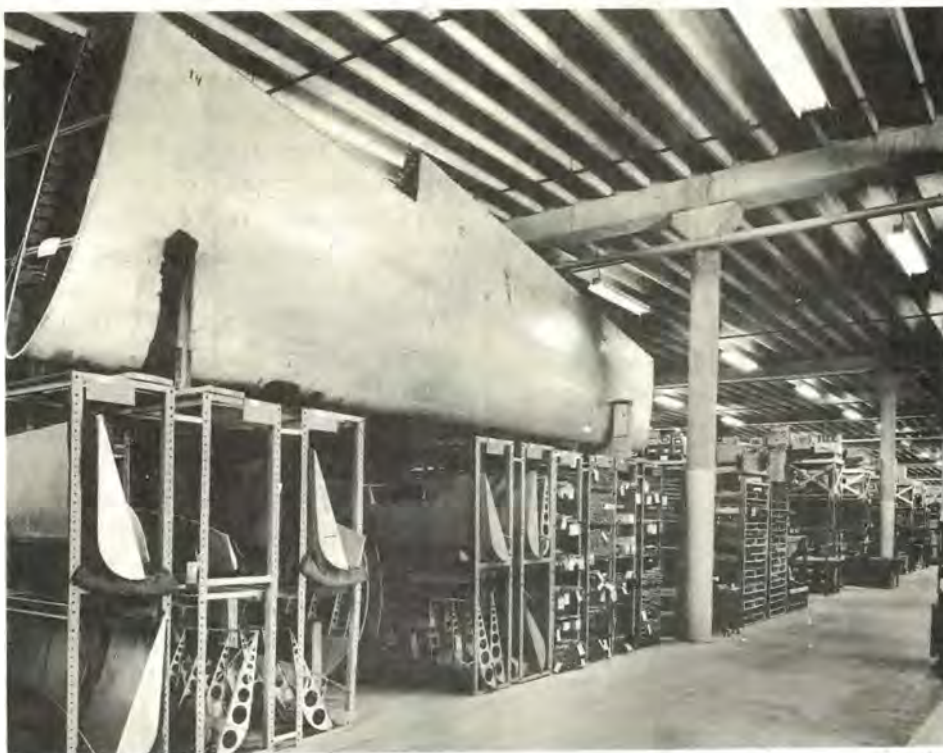
DC-3 wing and aileron assemblies. This is a good example of warehouse storage problems and space utilization.
