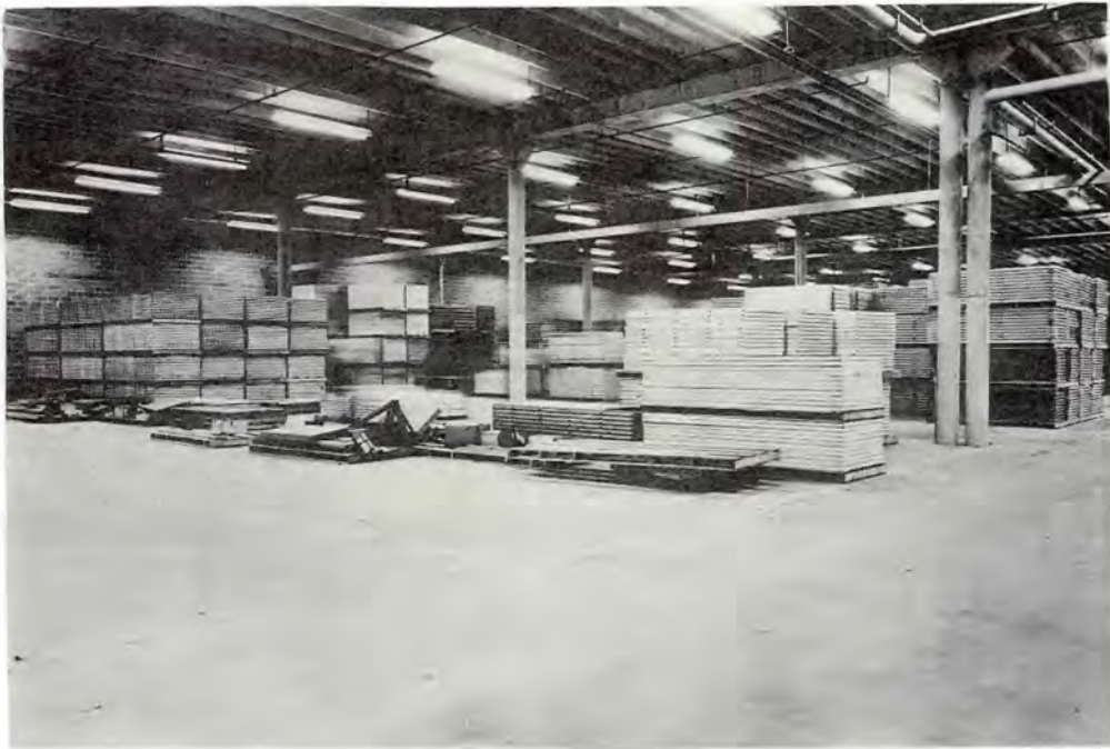
A PORTION of the Area "G" in the warehouse building where the Operations Section stores the wall panels for the pre-fabricated buildings that are used in most of the Air Navigation Facility sites. These panels are used to erect buildings which vary in length and width in multiples of four feet.
