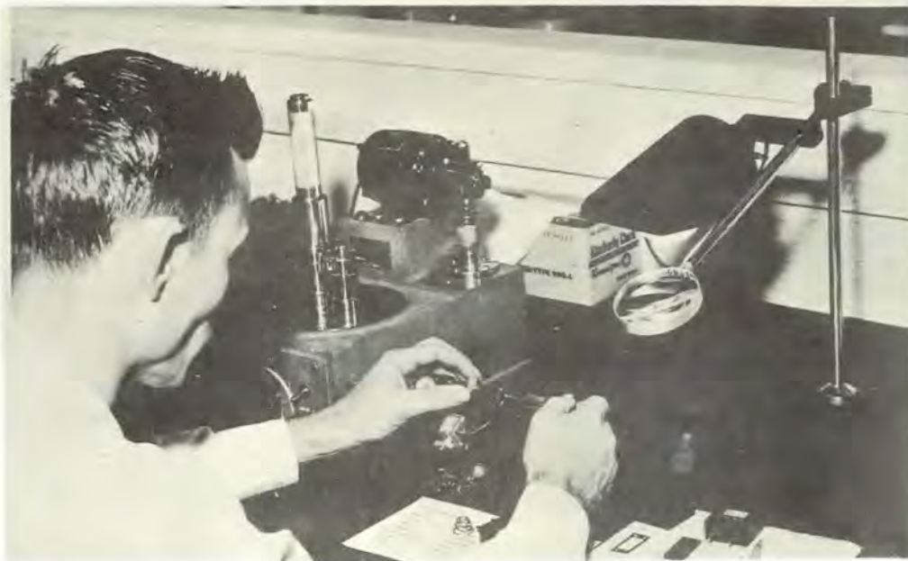
CRYSTAL TECHNICIAN Alfred Ray, Jr., is seen here very busy measuring a tiny piece of quartz capable of vibrating four and a half million times per second under appropriate conditions. This delicate piece of mineral is protected in service by a small fully enclosed case. Crystals are used in almost all of our aids to navigation because of their inherent stable vibrating qualities.
