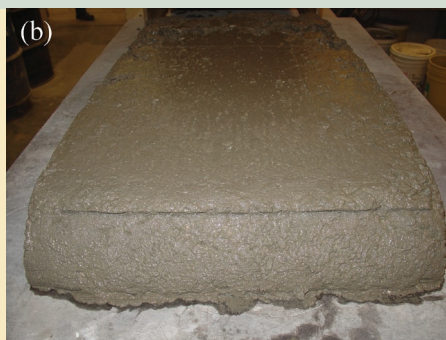
(a) The first photo shows consolidation and shape stability of a model pavement slab for a standard slipform mix. The rough pavement exhibits poor consolidation. (b) Consolidation and shape stability of a model pavement slab for an SF-SCC developed with fly ash. The bulging sides indicate poor shape stability, but the smooth surface indicates good consolidation. (c) Consolidation and shape stability of a model pavement slab for an SF-SCC developed with clay and fly ash. The smooth surface and straight sides indicate both acceptable consolidation and shape stability. Photos: ACBM.
