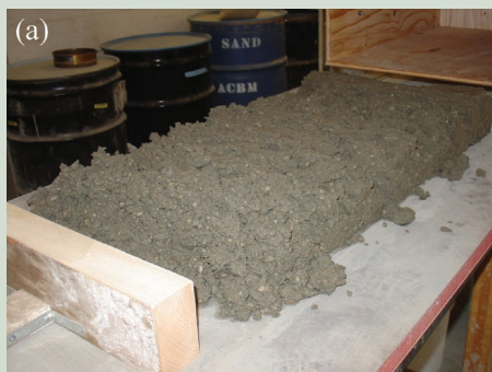
(a) The first photo shows consolidation and shape stability of a model pavement slab for a standard slipform mix. The rough pavement exhibits poor consolidation. (b) Consolidation and shape stability of a model pavement slab for an SF-SCC developed with fly ash. The bulging sides indicate poor shape stability, but the smooth surface indicates good consolidation. (c) Consolidation and shape stability of a model pavement slab for an SF-SCC developed with clay and fly ash. The smooth surface and straight sides indicate both acceptable consolidation and shape stability. Photos: ACBM.
