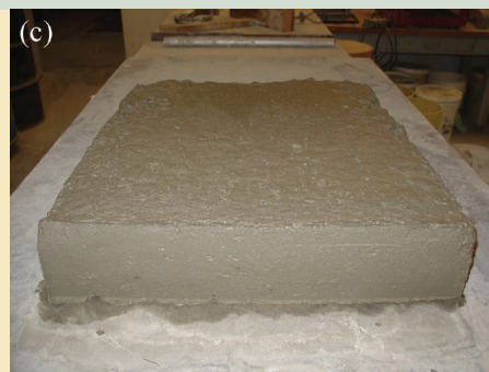
(a) The first photo shows consolidation and shape stability of a model pavement slab for a standard slipform mix. The rough pavement exhibits poor consolidation. (b) Consolidation and shape stability of a model pavement slab for an SF-SCC developed with fly ash. The bulging sides indicate poor shape stability, but the smooth surface indicates good consolidation. (c) Consolidation and shape stability of a model pavement slab for an SF-SCC developed with clay and fly ash. The smooth surface and straight sides indicate both acceptable consolidation and shape stability. Photos: ACBM.
