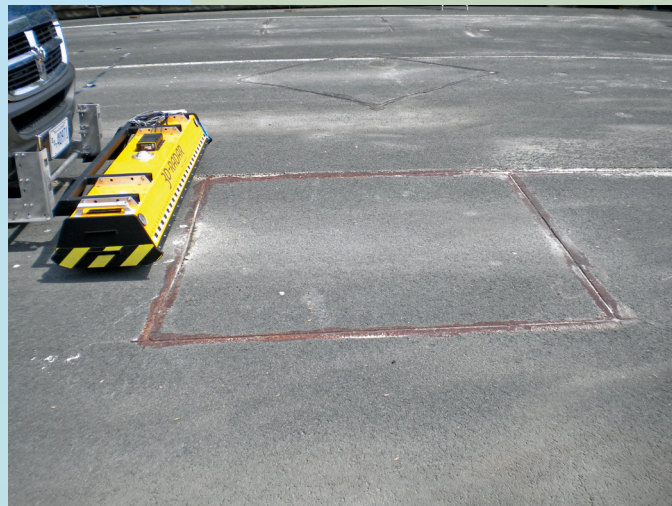
Researchers are using the Advanced Pavement Evaluation system (mounted on the front of the van) to scan loop wires embedded in the pavement. The loop wires are diamond-shaped (left) and square-shaped (right), as indicated by the adhesive-filled sawcut marks in the pavement surface.
