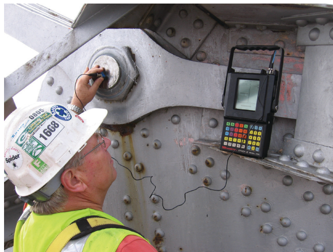
A bridge inspector conducts ultrasonic tests on a steel bridge.
