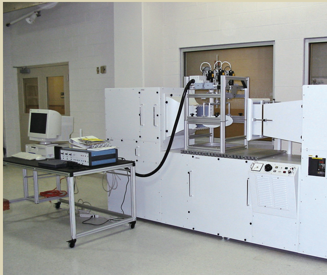
The small, closed-circuit wind tunnel at the lab is shown with a shaker apparatus installed in the test section at the photo's center. A bridge section model is installed in the shaker for forced vibration testing.
