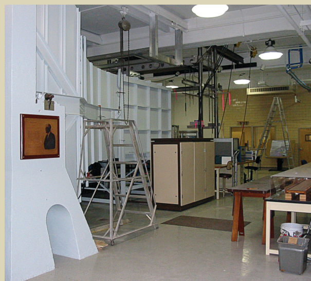
In the large, open-circuit wind tunnel (far left) in FHWA's Aerodynamics Laboratory at TFHRC, smooth and turbulent wind conditions are simulated during static and dynamic testing of structural models.
