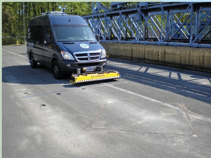
Researchers are using the Advanced Pavement Evaluation system (mounted on the front of the van) to scan loop wires embedded in the pavement. The loop wires are diamond-shaped (left) and square-shaped (right), as indicated by the adhesive-filled sawcut marks in the pavement surface.
