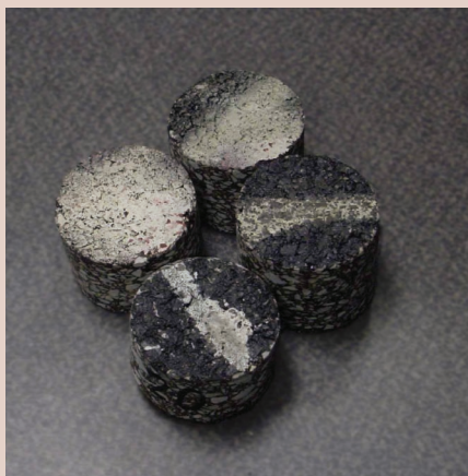
Shown here are asphalt core samples that OIG special agents seized as evidence from a project on Page Avenue in St. Louis, MO. The double-marked cores (top left) were from the job site, whereas the nondouble-marked cores (lower right) were allegedly substituted.
