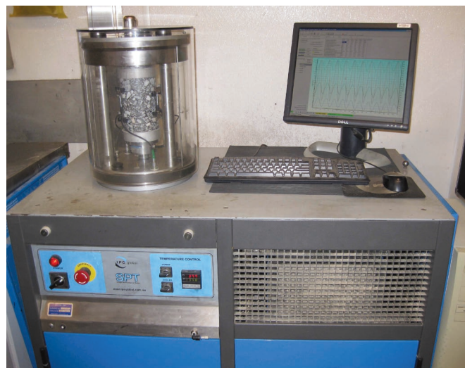
Shown here, the new asphalt mixture performance tester is used to evaluate Superpave mixtures.
