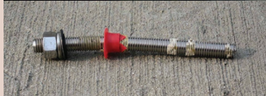
This anchor bolt dislodged from the ceiling of the I-90 tunnel when the epoxy adhesive failed.
