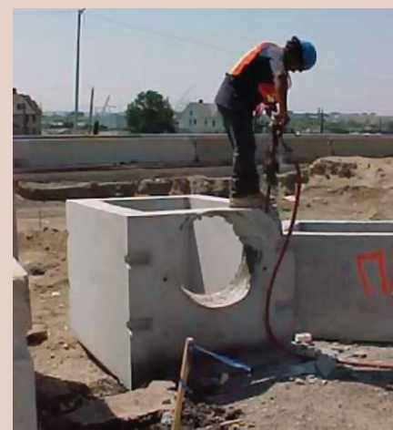
A State inspector destructively tests a precast concrete catch basin to determine whether it meets contract specifications for a reconstruction project on I-95 in Bridgeport, CT.
