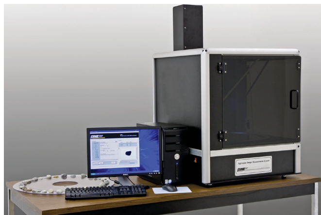
AIMS2, developed through an FHWA Technology Partnership grant, includes a computer and monitor, the AIMS software, and the image acquisition hardware, as shown here.
