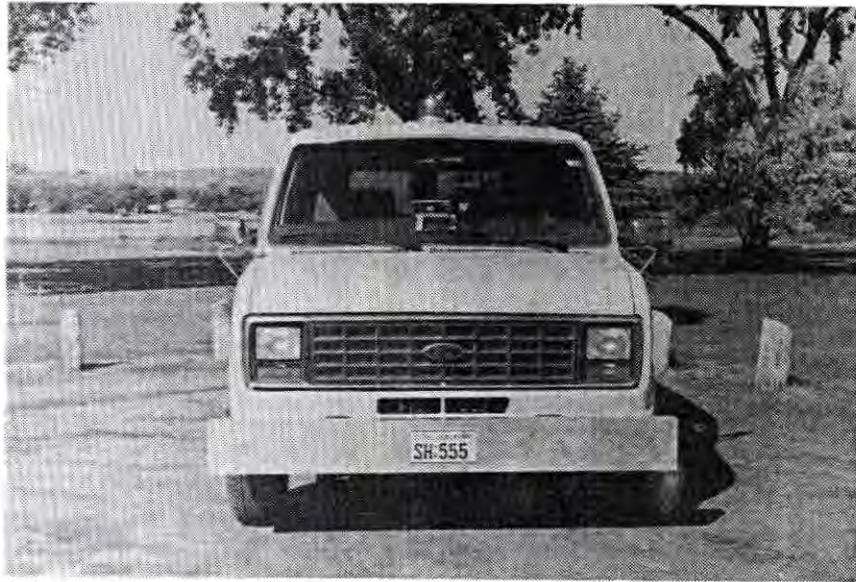
Figure 2: South Dakota Road Profiler
