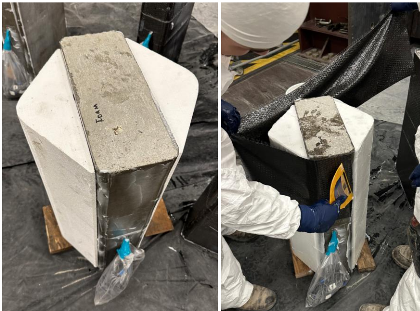
Figure 14 Preparing geofoam-profiled FRP jacket.
