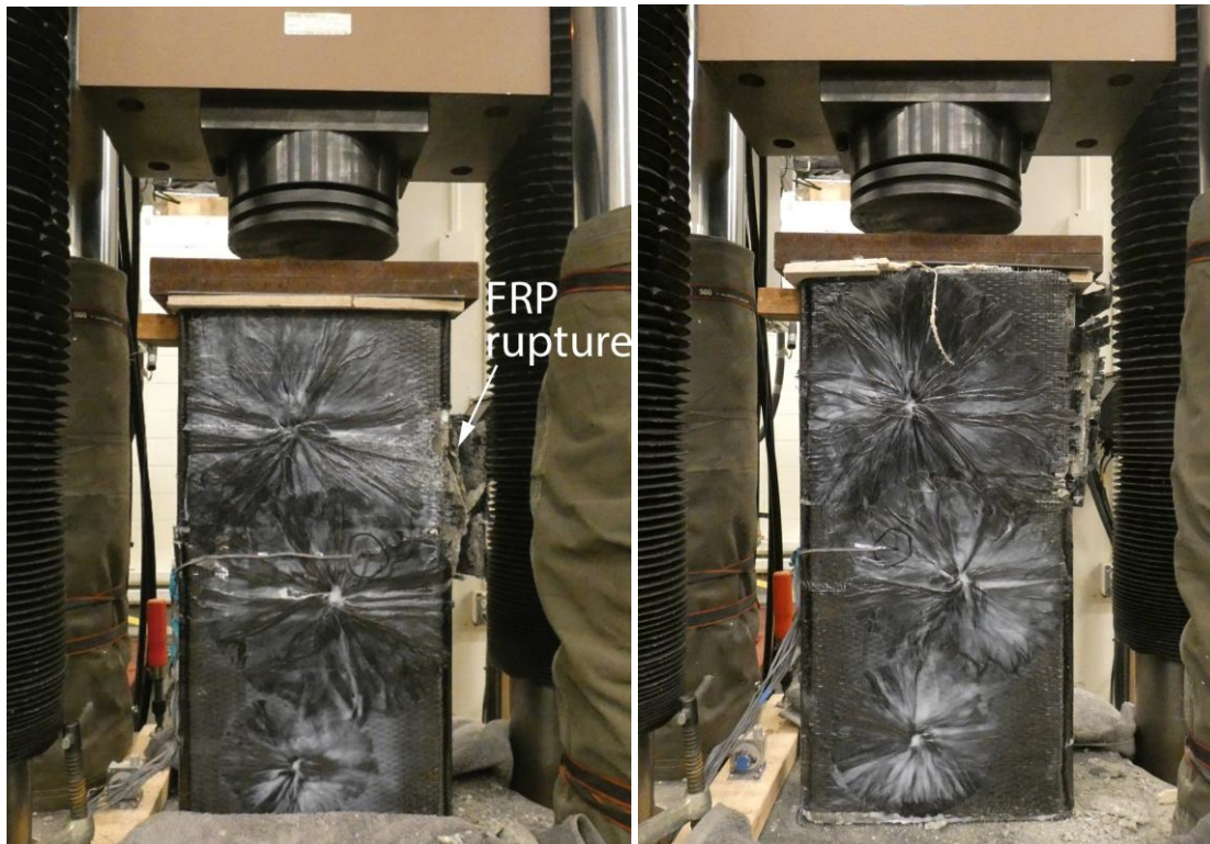
Figure 30 Failure mode of Group 3 columns.
