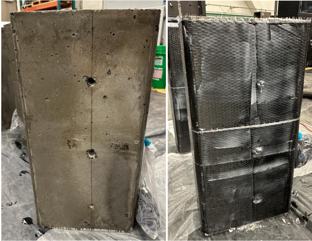
Figure 11 Drilling anchor holes and wet layup of FRP over the holes.
