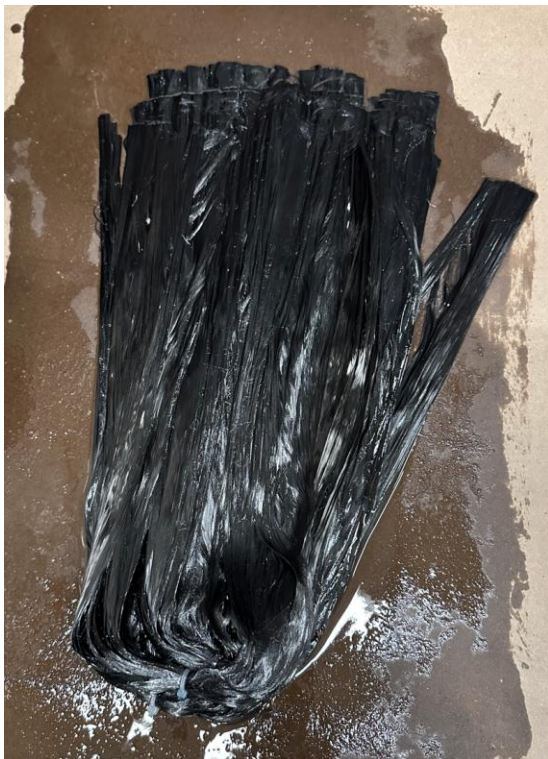
Figure 12 Preparing FRP anchor with resin.
