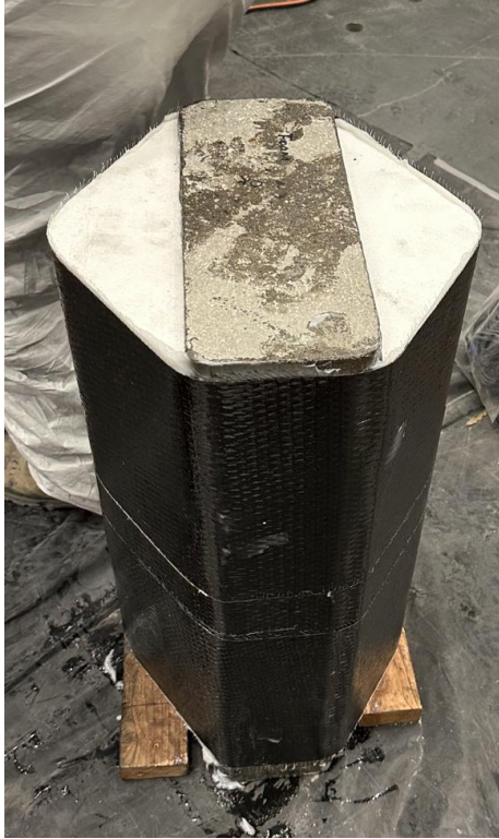
Figure 15 Columns with geofoam-profiled FRP jacket.
