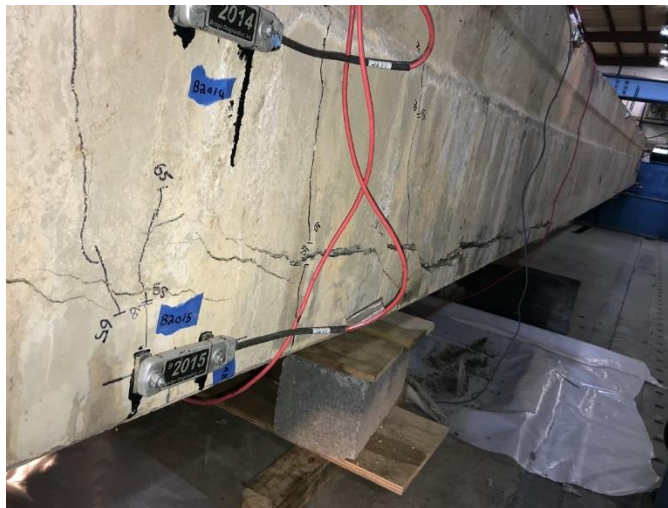
Figure 63. Propagation of the Cracks of the East Side of Box Beam 1 During the Test
