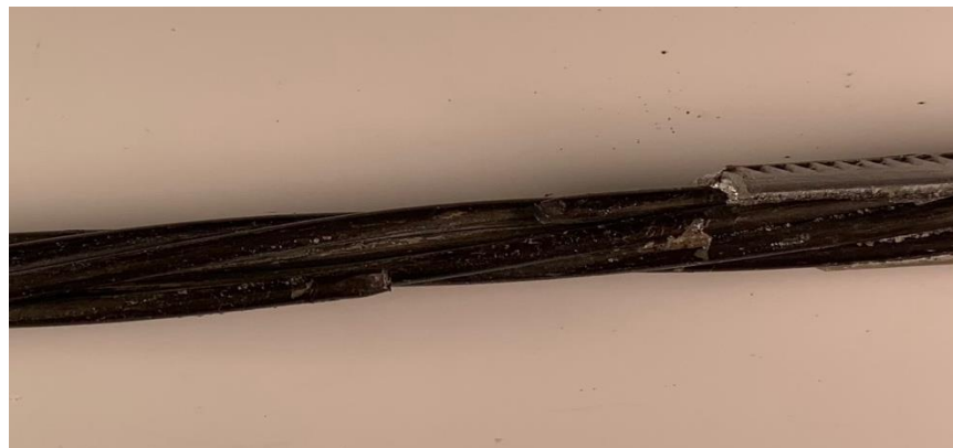
Figure 83. Strand Taken from I-Beam 7 after Testing
