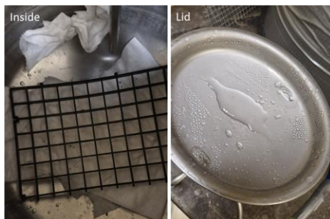
Figure 7.4. Water released from six mortar cubes during carbonation process
