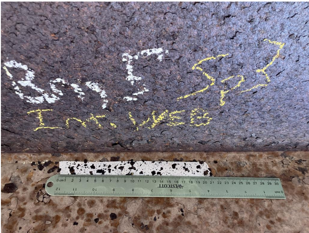
Figure 69. Photograph of a tape test conducted on the web of an interior beam belonging to No. 606750, dated December 12, 2023, from NBI inspection records.
