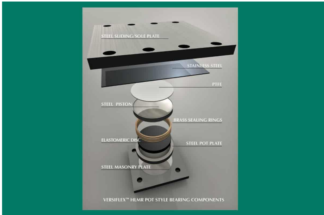
Figure 95. Exploded view of pot bearing (D.S. Brown, 2022)
