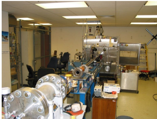
Figure 5.8: Single Stage Gas Gun Set-Up at NASA-Glenn Research Center.
