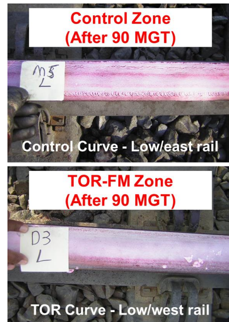
Figure 6: Union Pacific Tehachapi trial. RCF development at 90 MGT – significant reduction in low rail RCF for the “TOR FM zone” compared to the “control zone”.
