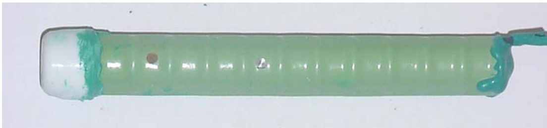
Figure 5.11 – Bare ECR anode bar, at 15 weeks, showing corrosion products that formed at drilled holes.
