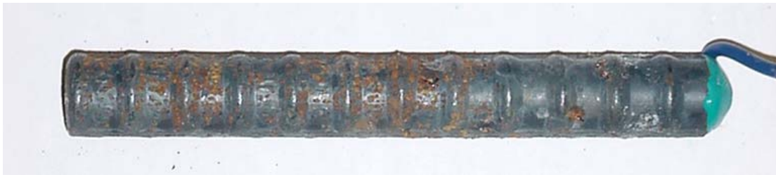
Figure 5.9 – Bare conventional anode bar, at 15 weeks, showing corrosion products that formed below the surface of the solution.
