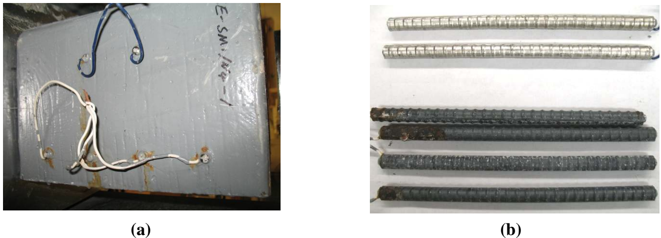
Figure 5.28 – Southern Exposure Specimen SMI/Conv.-1. (a) Specimen and (b) top bars (top) and bottom bars (bottom) at conclusion of corrosion test
