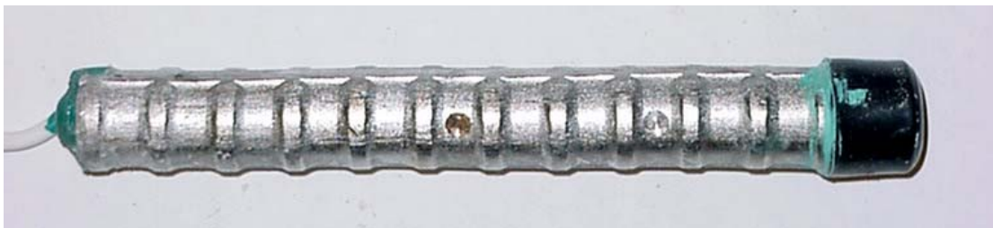
Figure 5.14 – Bare SMI-d anode bar from 1.6 m ion salt solution, at 15 weeks, showing corrosion products that formed at penetrations through the cladding.
