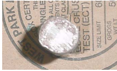
Figure 5.15 – SMI-nc anode bar after removal of mortar, at 15 weeks, showing corrosion products that formed at the unprotected end.
