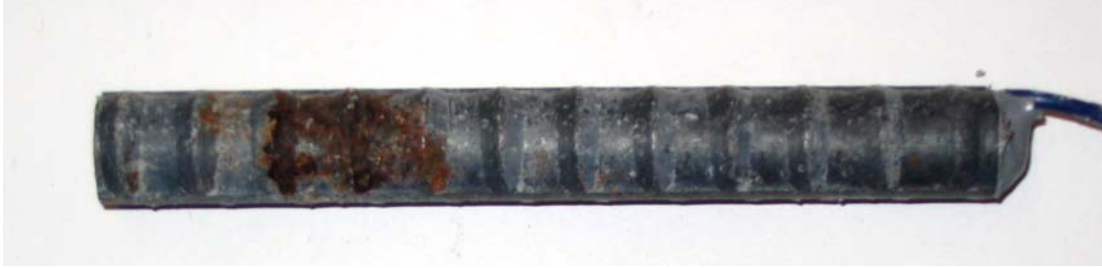
Figure 5.12 – Conventional anode bar after removal of mortar, at 15 weeks.
