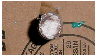
Figure 5.13 – Bare SMI-nc anode bar from 1.6 m ion salt solution, at 15 weeks, showing corrosion products that formed at the unprotected end.
