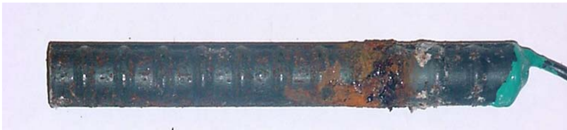
Figure 5.10 – Bare conventional anode bar, at 15 weeks, showing corrosion products that formed at contact points between the bar and plastic lid.
