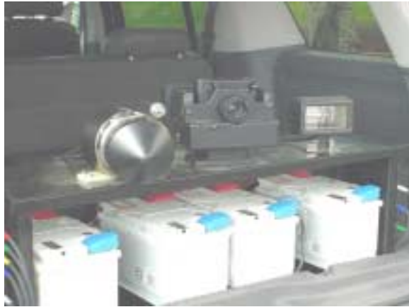
Figure 1 Antenna, camera, flash and batteries installed in rear of vehicle.
