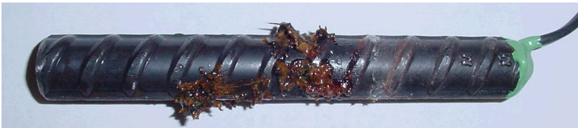
Figure 5.5 – Bare MMFX anode bar from group MMFX(2), at 15 weeks, showing corrosion products that formed below the surface of the solution.
