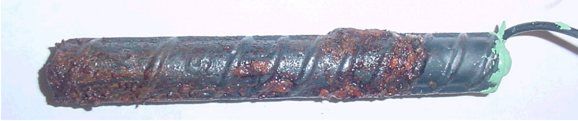
Figure 5.3 - Bare conventional N3 anode bar, at 15 weeks
