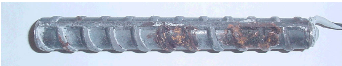
Figure 5.11 - MMFX anode bar after removal of mortar, at 15 weeks.
