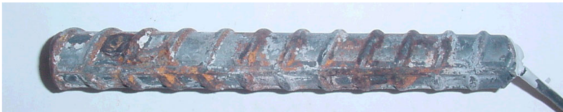
Figure 5.10 - Conventional N3 anode bar after removal of mortar, at 15 weeks.
