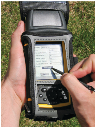
A researcher demonstrates the handheld data collector developed for the Roadkill Observation Collection System project.
