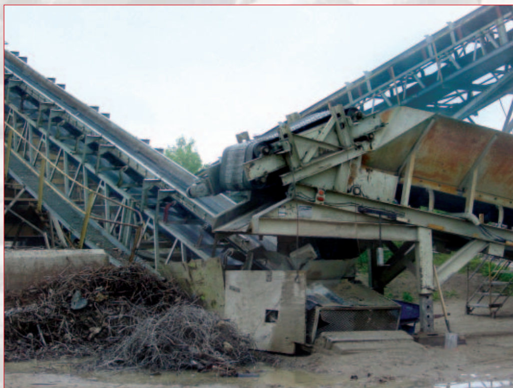
A magnetic belt removes the remaining metal from crushed concrete rubble.
