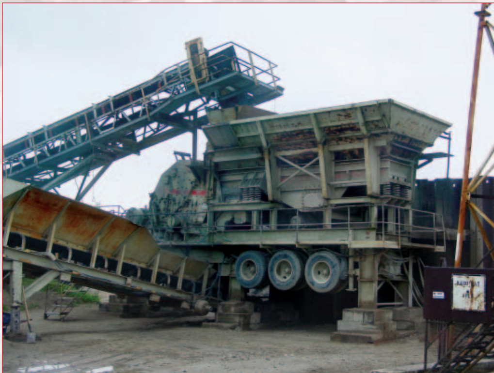
An impact crusher is used to break concrete rubble.
