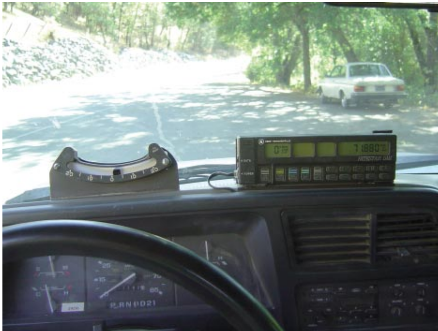
A ball bank indicator and distance measuring instrument are mounted on a car dash in the line of sight.
