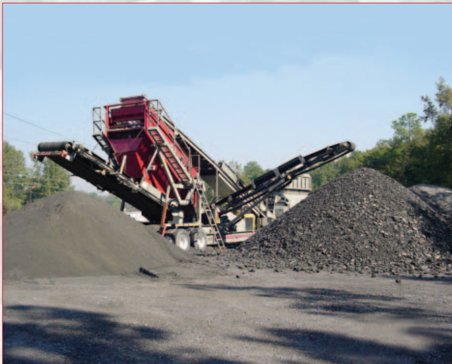
This equipment is used to fractionate (separate) RAP.
