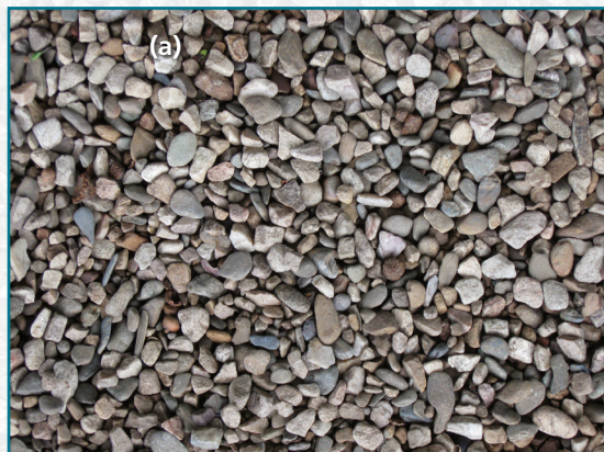
Shown here are examples of natural aggregates used in construction: (a) natural gravel often used as coarse aggregate in concrete, (b) crushed stone coarse aggregate typically used in asphalt mixtures in paving and in concrete, and (c) a compacted crushed stone layer used as granular base material. Photos: Richard Meininger, FHWA.
