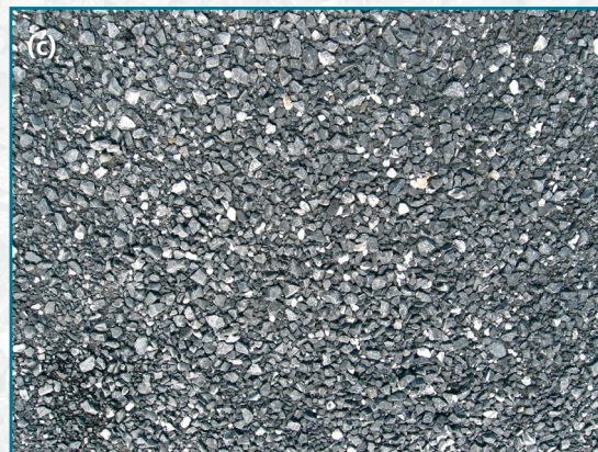
Shown here are examples of natural aggregates used in construction: (a) natural gravel often used as coarse aggregate in concrete, (b) crushed stone coarse aggregate typically used in asphalt mixtures in paving and in concrete, and (c) a compacted crushed stone layer used as granular base material. Photos: Richard Meininger, FHWA.
