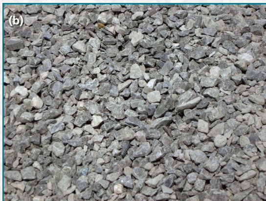
Shown here are examples of natural aggregates used in construction: (a) natural gravel often used as coarse aggregate in concrete, (b) crushed stone coarse aggregate typically used in asphalt mixtures in paving and in concrete, and (c) a compacted crushed stone layer used as granular base material. Photos: Richard Meininger, FHWA.
