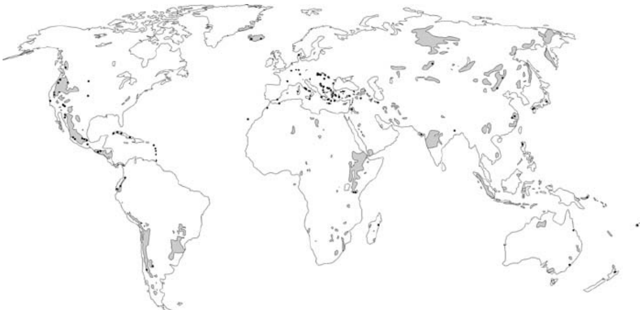
Figure 3.2: Global distribution of volcanic rocks (shaded areas) and natural pozzolan deposits (dots).
