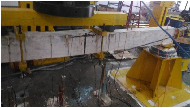
Fig. 6 Failure of the retrofitted specimen REP2-2
