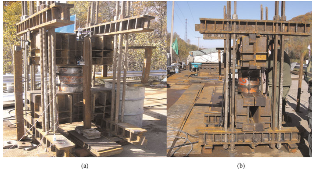
Fig. 12 Load test devices, including the strain and the deflection dial gauges. (a) Isometric view; (b) side view
