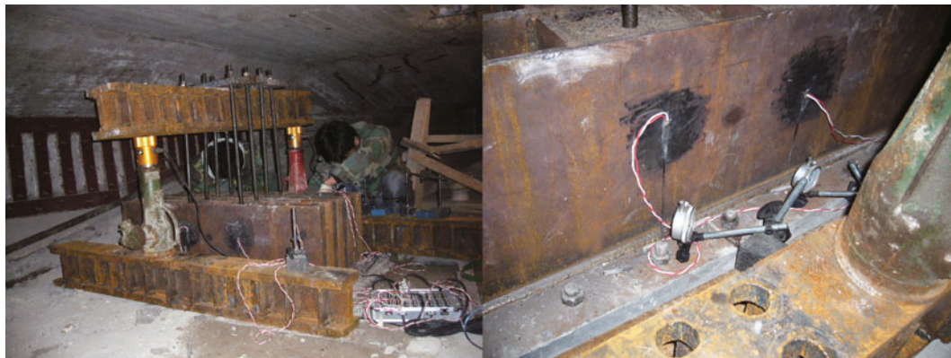
Fig. 16 Dial gauge location
