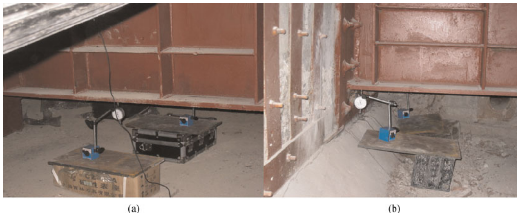
Fig. 6 Locations of the deformation dial gauges on the cross beam. (a) At mid-span; (b) at end-span
