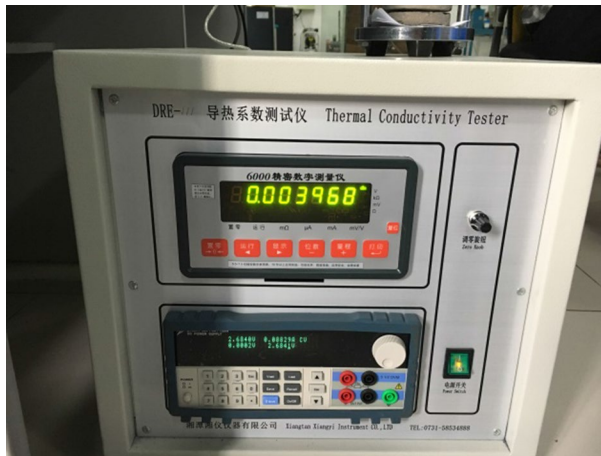
Fig. 3 DRT-III thermal conductivity tester
