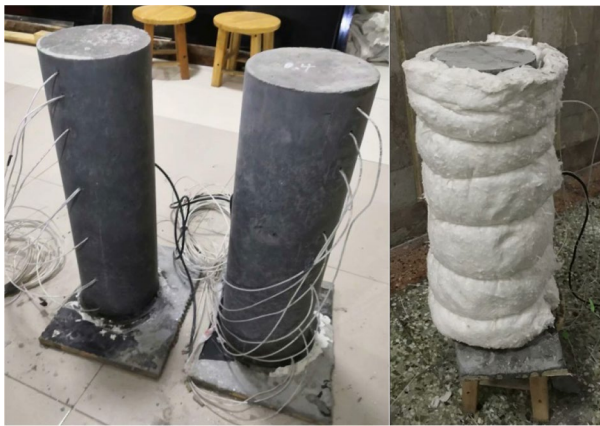
Fig. 5 Concrete samples and the sample with insulation
