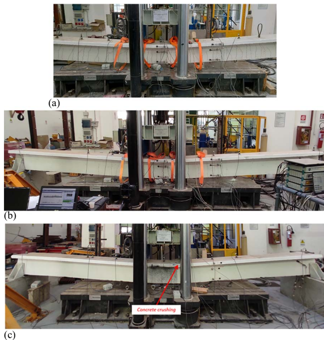
Fig. 12. Failure configuration of the specimens: (a) T3 (B-LP) (B); (b) T4 (U-LP); and (c) T5 (PB-M-HP).
