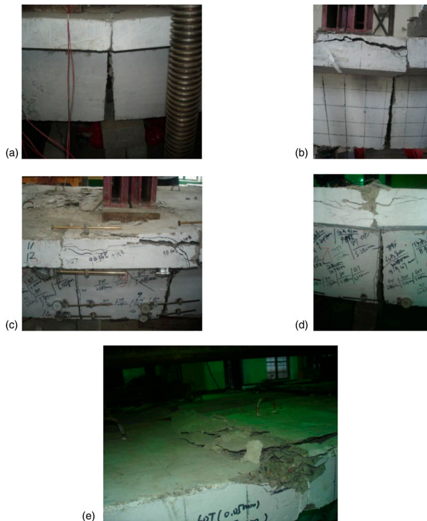
Fig. 9. Failure modes of each segmental box girder: (a) flexural failure of SPCBG1; (b) flexural and shear failure of SPCBG2; (c) flexural and shear failure of SPCBG3; (d) flexural failure of SPCBG4; (e) flexural failure of SPCBG5
