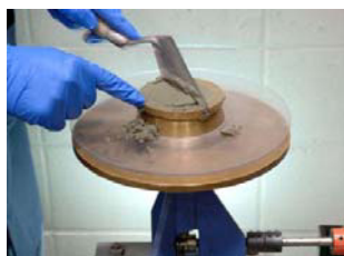
Fig. 5. Flow-table test procedure.
