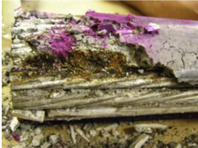
ID-15.6. Corrosion of a strand embedded in deficient grout. Pink colour shows the Ph indicator (phenolphthalein) sprayed on the grout surface (Lau and Lasa, 2016).
