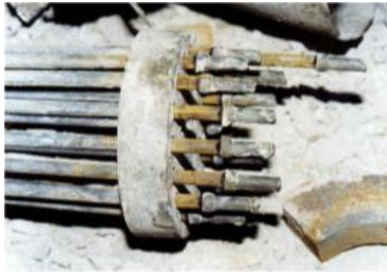
Figure 3.3.3. Corrosion of wires at anchorage plate in I-94 Bridge over US 81 (ID-30) (Dickson et al, 1993).
