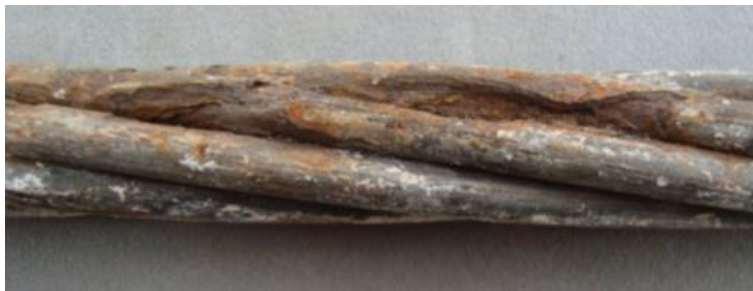
ID-18.3. Example of corrosion attacks on a prestressing strand in contact with the whitish segregated grout (Bertolini and Carsana, 2011).
