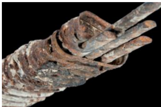
ID-19.6. Remaining bituminized roofing on a completely failed, non-grouted and heavily corroded tendon (Helmerich and Zunkel, 2014).
