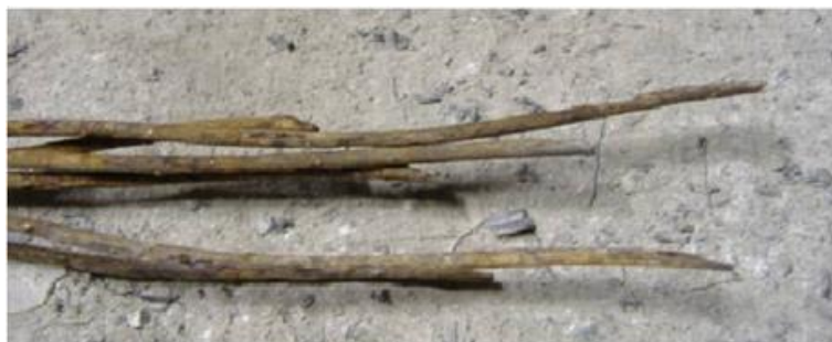
ID-18.4. Example of failed wires in a prestressing strand in contact with the whitish segregated grout (Bertolini and Carsana, 2011).
