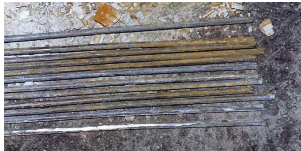
ID-30.2. Typical minor surface corrosion seen on post-tensioning wires removed from duct. No pitting or fractures were noted (Dickson et al, 1993).
