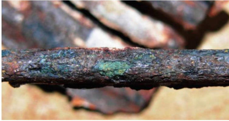
ID-3.4. Prestressing strand with corrosion products including dark-green-coloured rust (Papè and Melchers, 2011).
