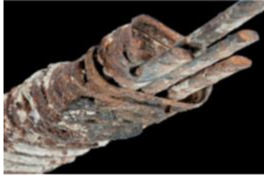
Figure 3.3.11. Remaining bituminized roofing on a completely failed, non-grouted and heavily corroded tendon in Berlin Congress Hall (ID-19) (Helmerich and Zunkel, 2014).
