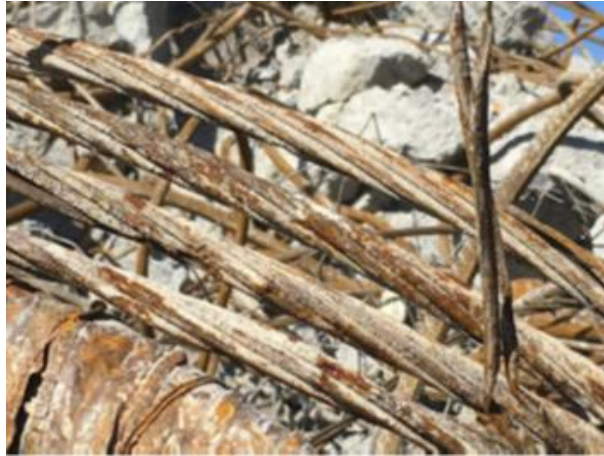
ID-6.9. Pitting corrosion of prestressing tendons (Morgese et al, 2020).
