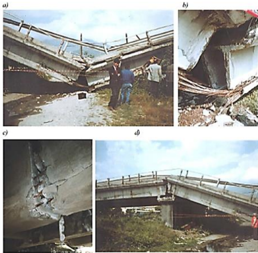
Figure 3.3.4. S. Stefano Viaduct (ID-2): a) collapse of the viaduct; b) slippage of cables; c) opening of joints; and d) rotation of the deck (Colajanni et al, 2016).
