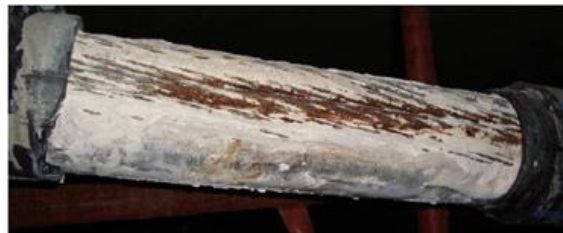
Figure 4.2.2.2. Example of whitish segregated grout embedding corroding strands in an Italian bridge (ID-18) (Bertolini and Carsana, 2011).
