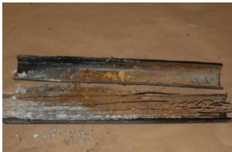
ID-15.3. Segment of failed tendon discovered in January 2011 with evidence of corrosion damage. Duct opened in laboratory during investigation (Ahern et al, 2018).
