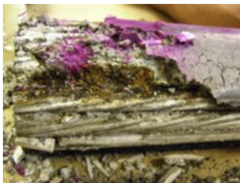
Figure 4.2.2.4. Corrosion of a strand embedded in deficient grout in Ringling Causeway Bridge (ID-15). Pink colour shows the pH indicator (phenolphthalein) sprayed on the grout surface (Lau and Lasa, 2016).
