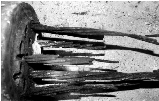
Figure 3 – Failed tendon-Niles Channel Bridge (June, 1999).
