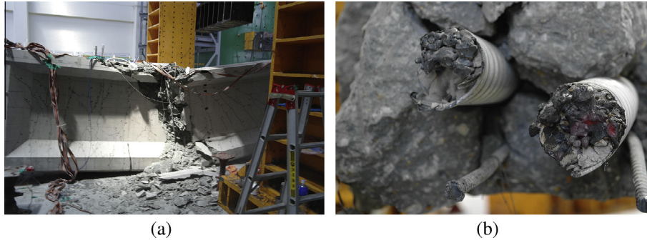
Fig. 5. Failure of the specimen HC: (a) failure mode; and (b) strands after failure.
