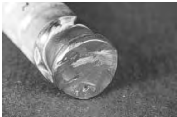
(f) Appearance of torch-cut end after wheel grinding and wheel brushing.
