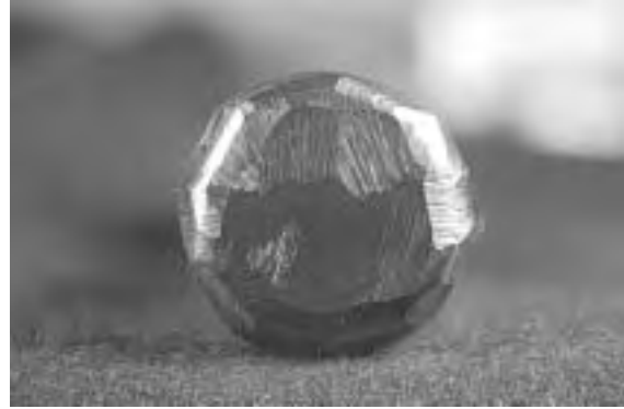
(b) Front view of specially cleaned bar end.
