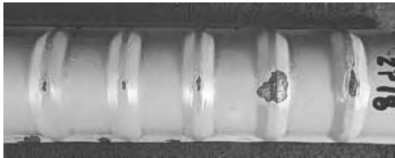
(b) Coating damage on transverse ribs.
