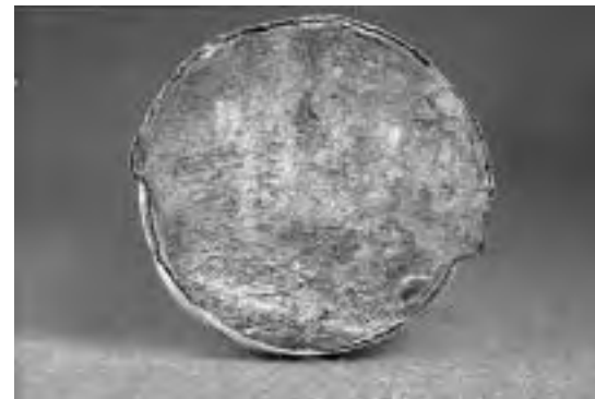
(f) Corrosion stage 4.
