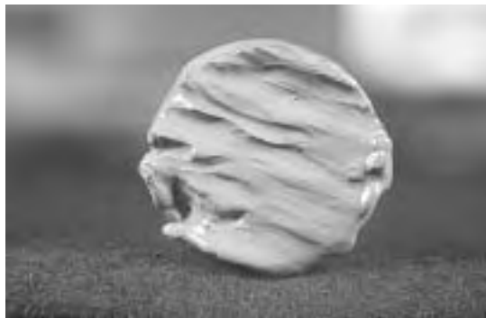
(e) Patched bar end (torch-cut) (IV).
