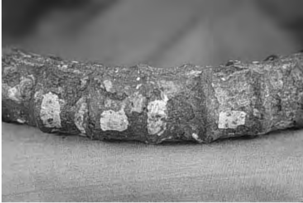
(a) Patched bar, outside bend.
