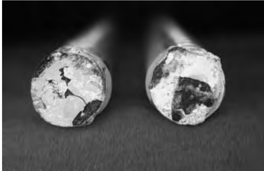
Figure 1.4 Patch at ends of spliced bars broke during autopsy, exposing a dark corroded surface after 4.3 years of exposure (beam study).
