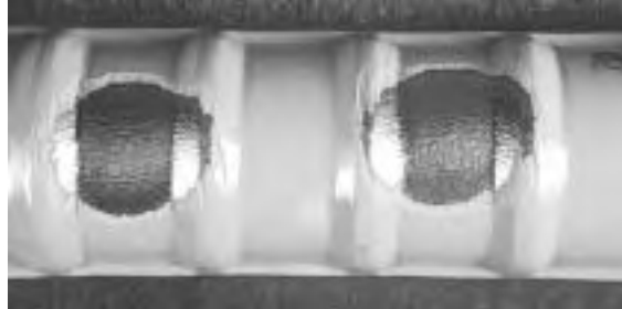
(d) Specially cleaned areas between bar deformations
