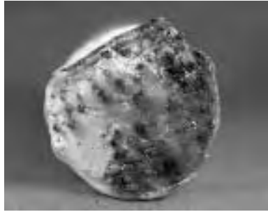
(a) Corrosion of patched end (shear-cut).
