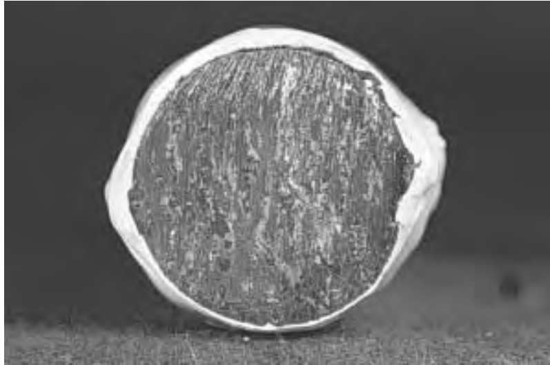
Figure 3.8 Good corrosion performance of bar end surface uncleaned before patching after 200 days of exposure to 3.5% NaCl solution.
