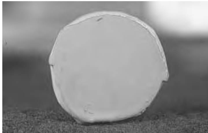
Figure 3.6 Visible steel due to very thin patch around perimeter edge on bar end.
