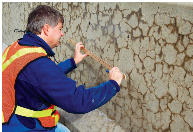
Dr. Benoit Fournier, an associate professor of geology at Laval University in Quebec, Canada, draws a grid on a concrete barrier to measure crack widths and determine the cracking index, which is used to estimate expansion and evaluate ASR damage.
