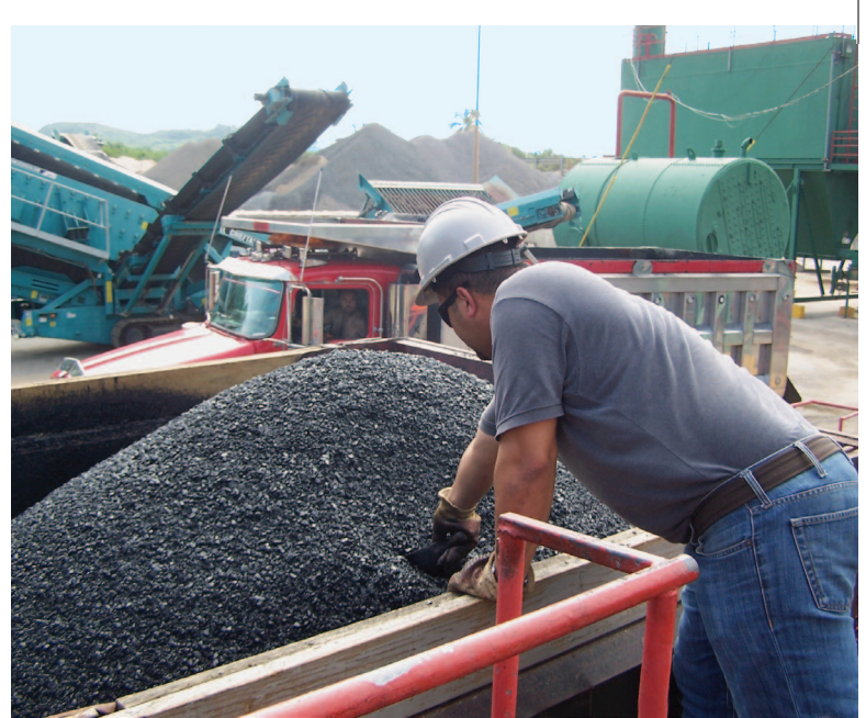
An inspector for the Puerto Rico Highway and Transportation Authority samples hot-mix asphalt from a truck for use in acceptance testing. Quality assurance is critical to meeting Federal and State requirements and is among the topics covered in the Federal-aid Essentials initiative.
