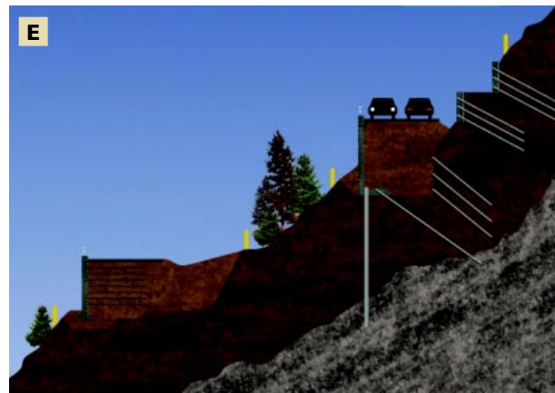
B. The process is repeated as the crew installs a second set of retaining walls into the hillside. Mass excavation is necessary to reach the bottom of the footing elevation for the walls that support the roadway.
