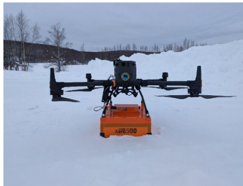
Figure 2. The Zone 500 radar is mounted to the DJI Matrice 300. The Radar and aircraft are seen after landing and between flights.
