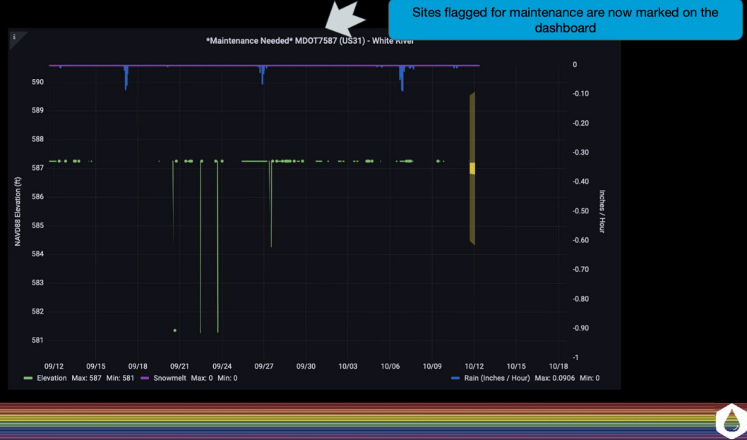
Figure 14. MDOT scour site data dashboard overview of features
