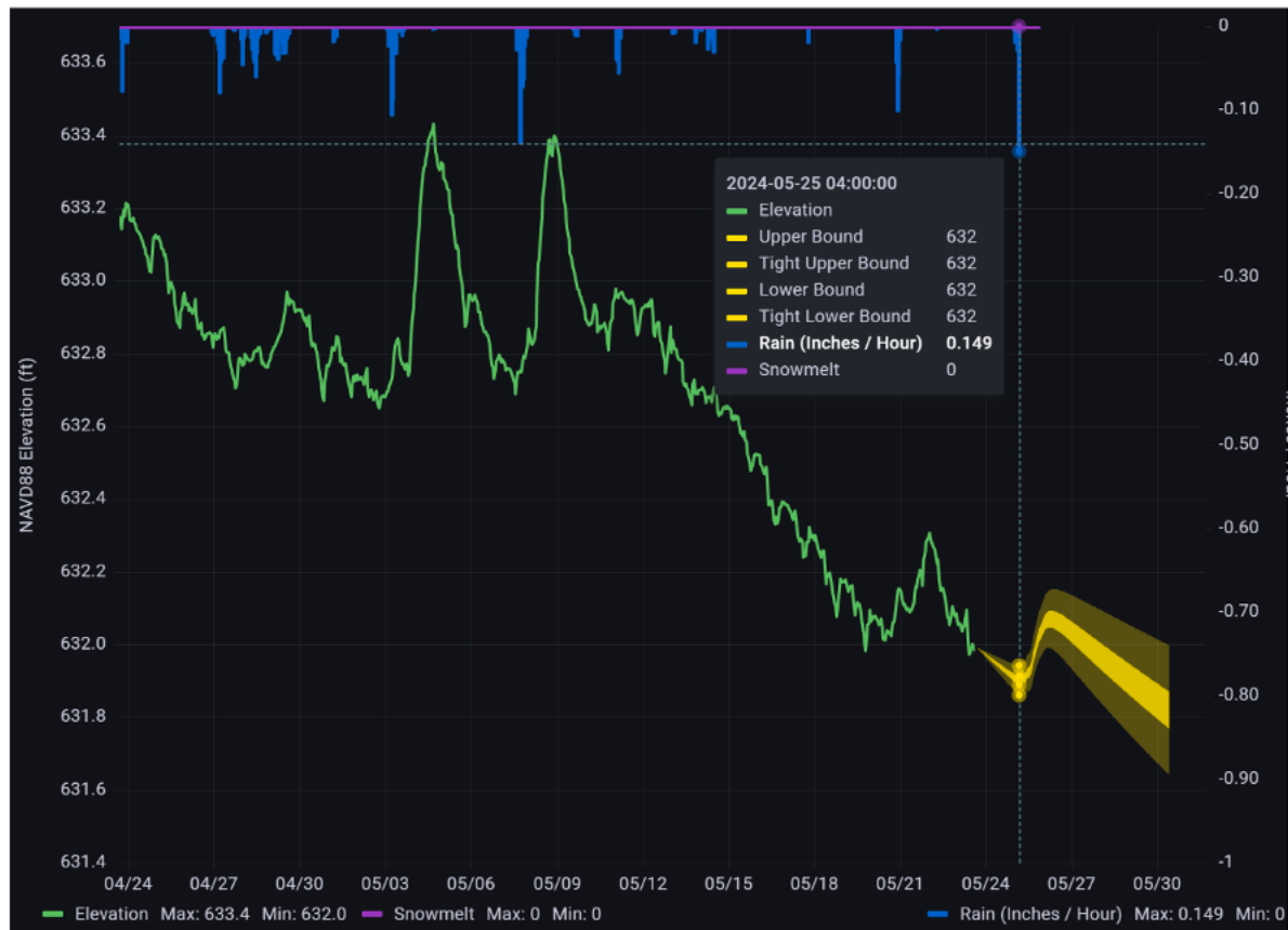
Figure 20. Sample forecasting support dashboard. Estimated snowmelt and rainfall (across all flow-distance regions) are indicated on top of the graph in purple and blue respectively. Historical water surface elevation is in green. Predictions with uncertainty estimates are provided in yellow.
