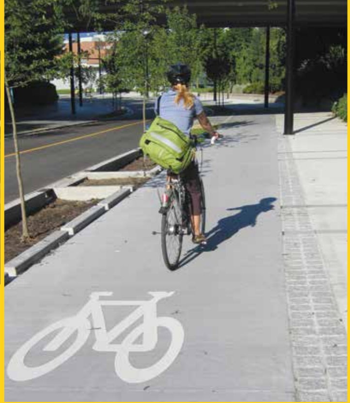
(Right) Small street trees in planter beds separate this bike lane from a street in Vancouver, British Columbia.
