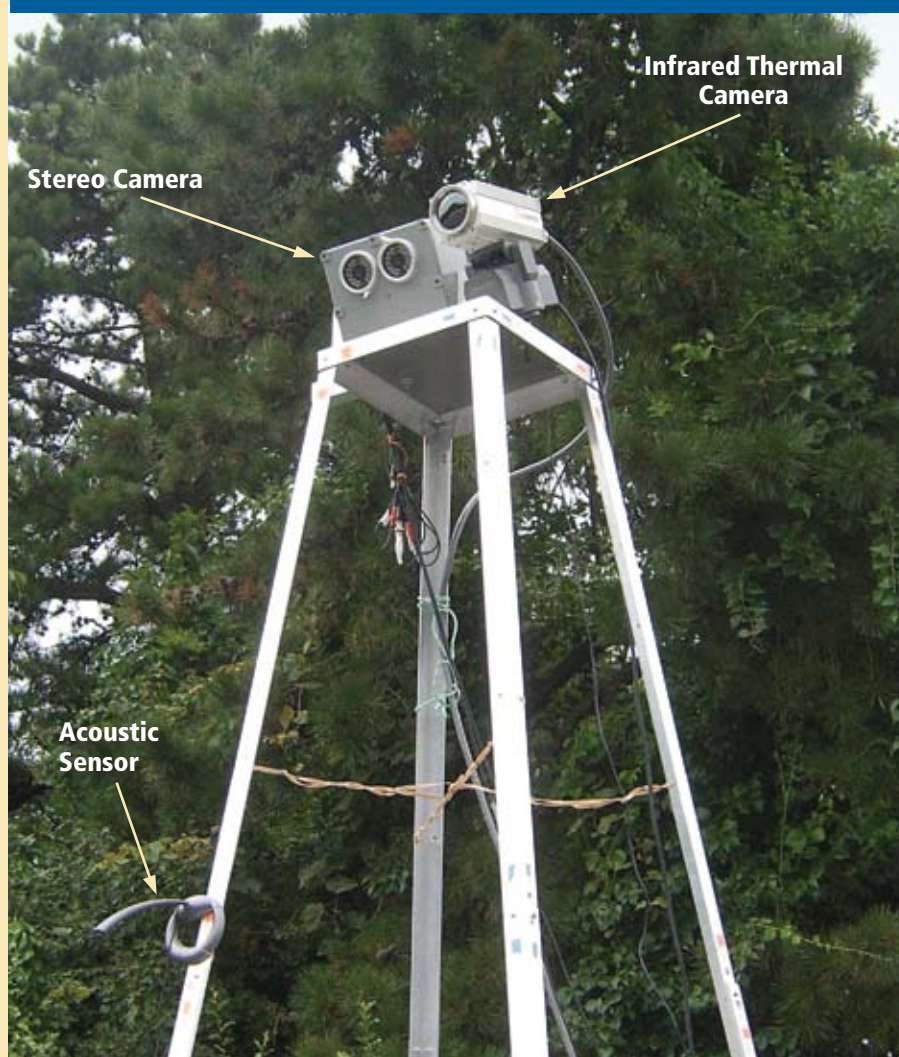
Shown here is a prototype motorcycle classifier, a multi-instrument sensor designed to detect cyclists at intersections. The sensor includes an infrared-visible light stereo camera (top left), an infrared thermal camera (right), and an acoustic sensor (below left).
