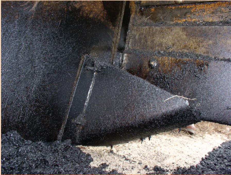
The Georgia wedge, shown here, is bolted onto the screed end gate.
