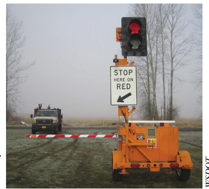
The ROBOFlagger, shown here, enables WSDOT flaggers to direct traffic from a safe distance away from the direct line of traffic.
