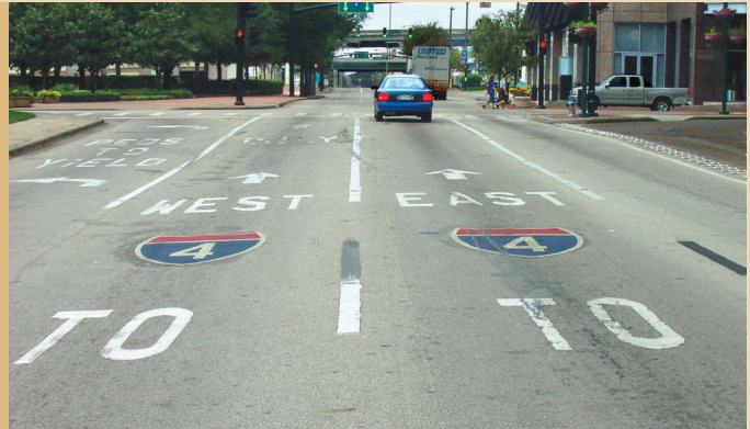
Traffic messages painted on the pavement in the driving lane, in full view of oncoming motorists, can provide an extra measure of communication with the driver. (Left) Motorists are alerted to an upcoming signal in Irvine, CA. (Right) Route markers on the pavement approaches to this intersection in Orlando, FL, help guide motorists to interstate access.
