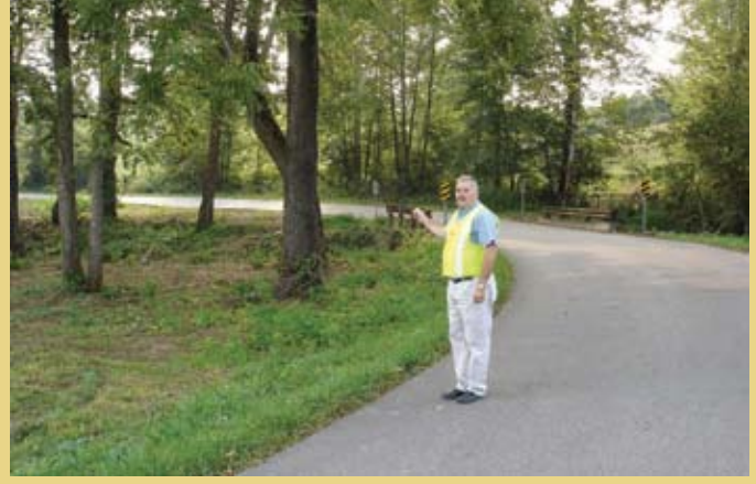
Between 2000 and 2005, 13 crashes were reported along this stretch of New Cummer Road in Morgan County. In 2005, county transportation officials dramatically improved safety along a bridge approach by clearing trees and brush to improve sight distances in the approach curve and installing Type 3 object markers to mark the bridge corners.
