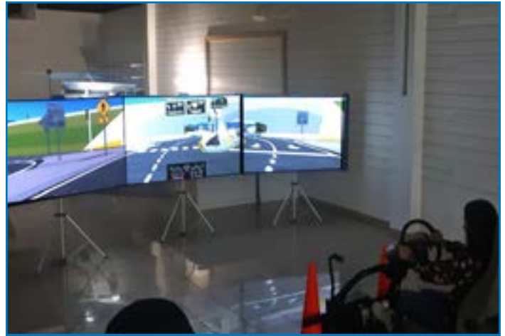
Driving simulation experiments helped inform the design of the new diverging diamond interchange as well as the communication plan.
