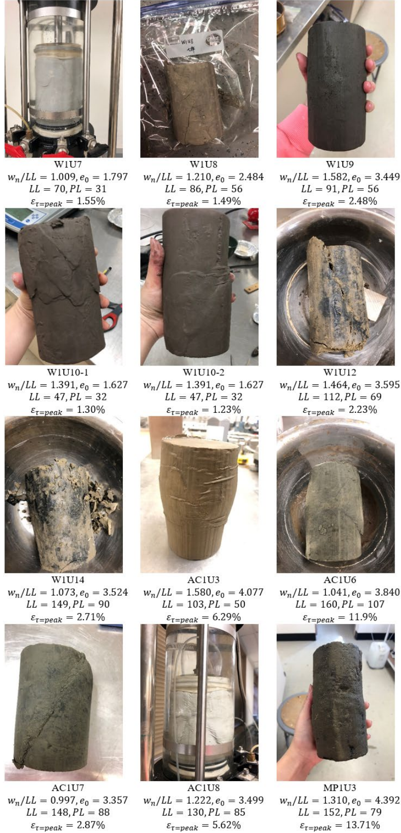
Figure 5.39: Failure patterns of all triaxial specimens and related physical properties
