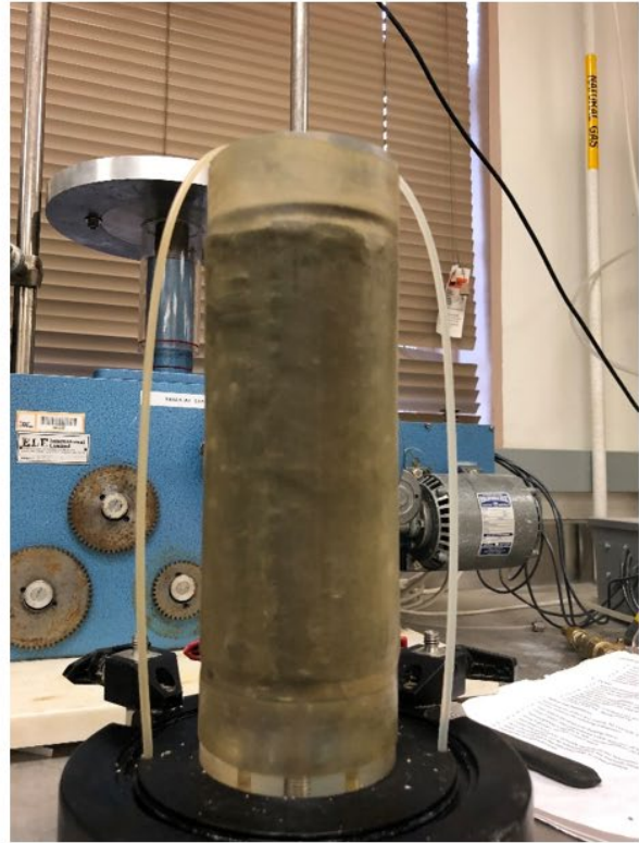
(b) Specimen enclosed in a membrane with top and bottom platens in place
