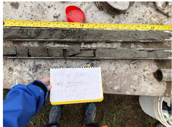
PC1N7, depth = 20.7m w_n = 137, LL = 141, PL = 75 \gamma = 12.2 \text{ kN/m}^3, G_s = 2.3 S_r = 93\%, FC = 95.2\%, (N_1)_{60} = 17.2
