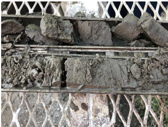
MP1N8, depth = 20.27m w_n = 125, LL = 148, PL = 69, SSA_{MB} = 28 m^2/g \gamma = 13 kN/m^3, G_s = 2.27 S_r = 99.6\%, FC = 94.7\%, (N_1)_{60} = 33.6
