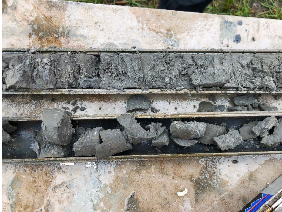
PC1N2, depth = 5.49m w_n = 92, LL = 114, PL = 49 \gamma = 12.9 \text{ kN/m}^3 FC = 87.6\%, (N_1)_{60} = 19.1
