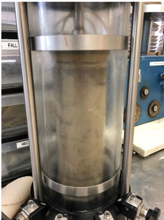
(c) Specimen mounted in the confining cell
