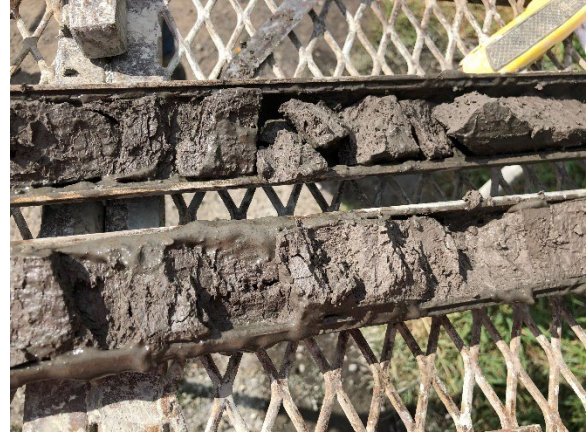
MP1N9, depth = 22m w_n = 120.4, LL = 130, PL = 81 \gamma_{calc} = 13.2 kN/m^3, G_s = 2.34 FC = 98.28\%, (N_1)_{60} = 28
