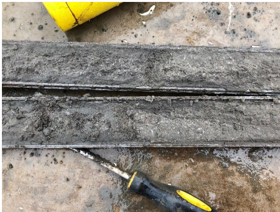
PC1N3, depth = 8.38m w_n = 109.6, LL = 109, PL = 75 \gamma = 13.2 \text{ kN/m}^3, G_s = 2.25 S_r = 98.5\%, FC = 97.9\%, (N_1)_{60} = 24.1
