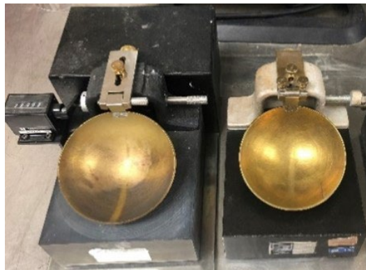
Figure 4.3: Casagrande cups (left: motorized; right: hand-operated)
