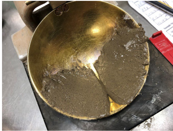
Figure 4.5: Example of diatomaceous soil sliding along the surface of the cup to close the groove.
