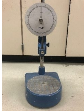
Figure 4.8: The fall cone device ( 30^\circ , 80g cone)
